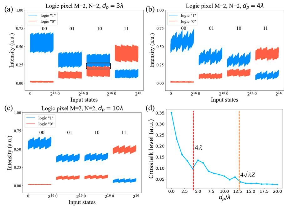
**Figure 3.** Effects on the logic-pixel mutual-interaction as the pixel-to-pixel gap  $d_p$  varies. The output of the center logic pixel for pixel gap  $d_p$  equals (a)  $3\lambda$ , (b)  $4\lambda$  and (c)  $10\lambda$ . (d) The crosstalk level of the parallel NAND operation versus pixel-to-pixel gap  $d_p$ .
