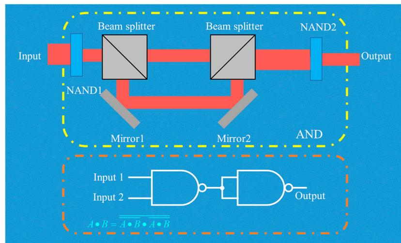
**Figure 6.** Generating AND gate with two cascaded NAND gates. Moving the Mirror 2 horizontally could combine two copies of the output from NAND-1 as the input for the second NAND-2.
