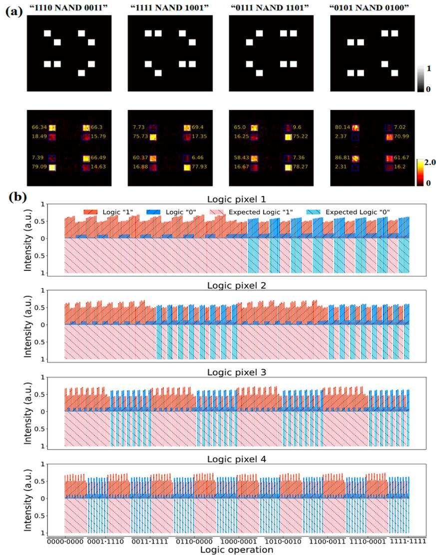
**Figure 2.** Logic operation for parallel NAND of the trained DONN. (a) Input-plane and corresponding output-plane intensity profiles for logic operations ‘1110 NAND 0011’, ‘1111 NAND 1001 = 0110’, ‘0111 NAND 1101 = 1010’, and ‘0101NAND 0100 = 1011’. (b) Parallel NAND logic operation outputs of all 256 inputs, in agreement with expectation states.
