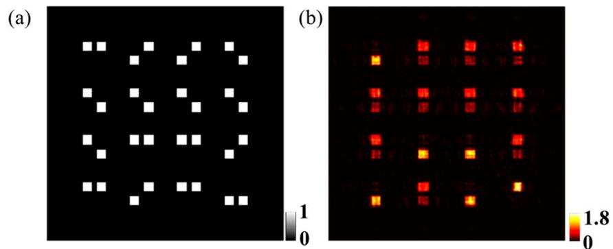
**Figure 4.** Example of a 16-bit parallel logic operation for ‘100111111101010 NAND 1110000001111110 = 0111111110010101’. (a) Input plane and (b) the corresponding output-plane intensity profiles.
