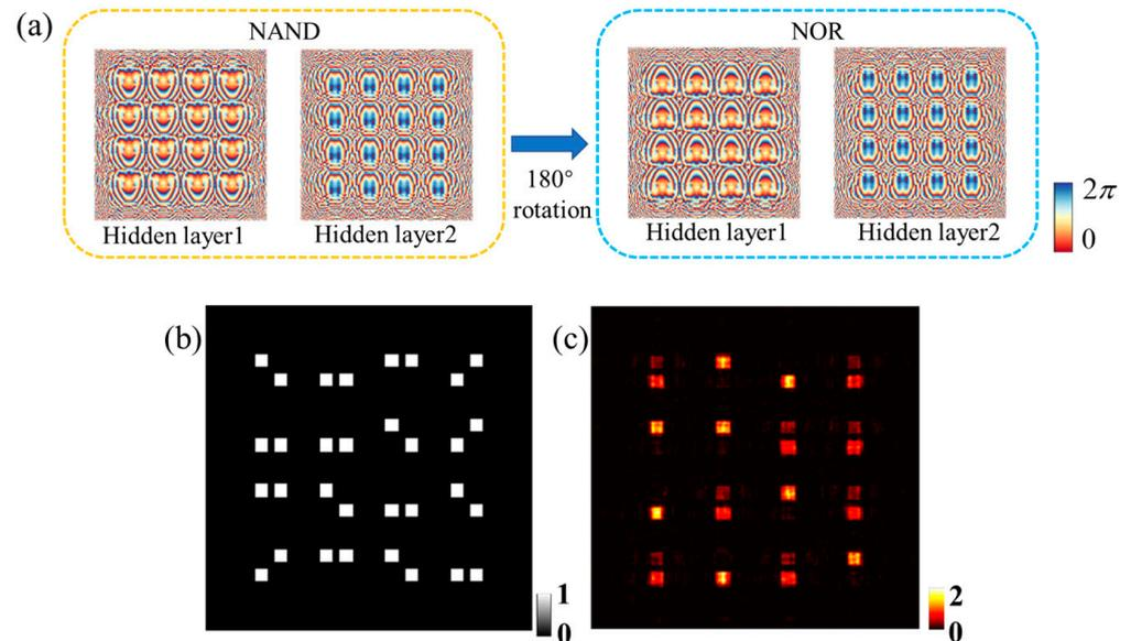
**Figure 5.** The 180° rotation of the DONN in a NAND operation turns the DONN into a NOR operation. (a) NAND (left) and NOR (right) DONN phase distributions of hidden layers. (b) Input-plane and (c) corresponding output-plane intensity profiles.
