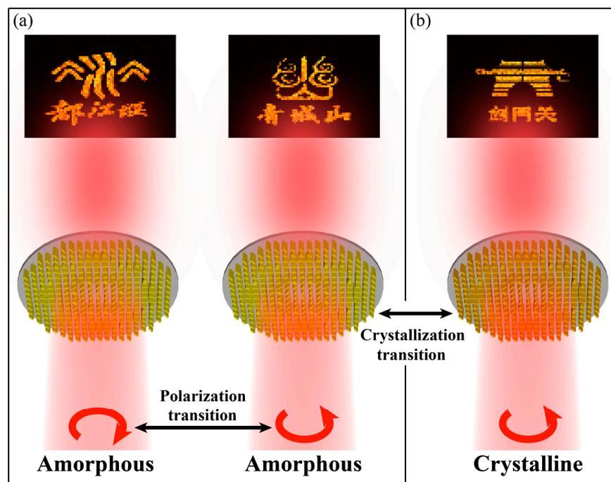
**Figure 1.** Schematic diagram of the proposed metasurface at different crystallization levels. (a) When GSST is in A-state, two different meta-holograms can be observed under RCP and LCP incidence. (b) When GSST changes to C-state, another meta-hologram can be observed and previous images in A-state are perfectly hidden.
