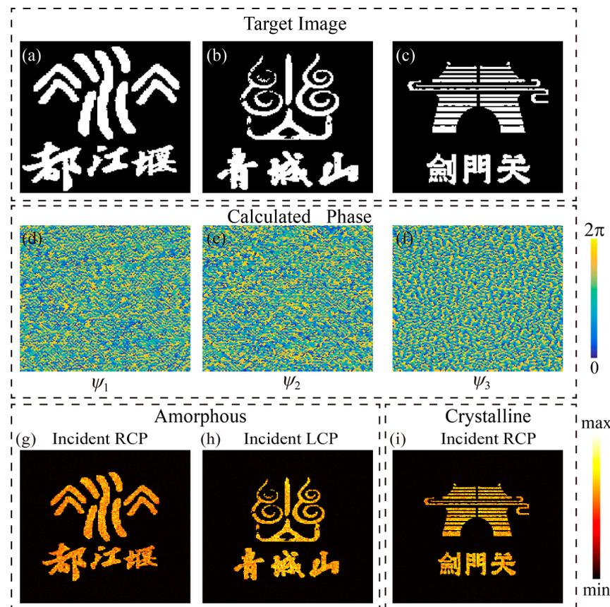
**Figure 5.** Multistate meta-hologram for information encryption. (a–c) Target images. (d–f) Calculated phase distributions based on GS algorithm. (g–h) Calculated far field results when GSST is in A-state under RCP (g) and LCP (h) incidences. (i) Calculated far field results when GSST is in C-state under RCP incidence.
