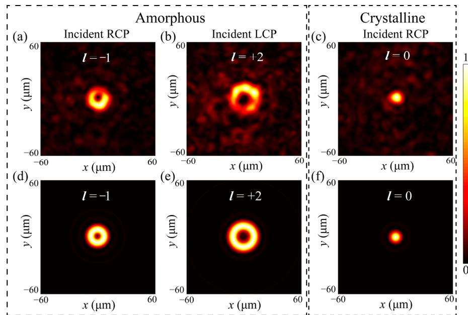
**Figure 4.** Simulated and theoretical performance of the designed multistate vortex beam generator. (a,b) The simulated electric field distributions when GSST is in A-state under RCP (a) and LCP (b) incidences. (c) The simulated electric field distributions when GSST is in C-state under RCP incidence. (d–f) The calculated results correspond to those in (a–c).
