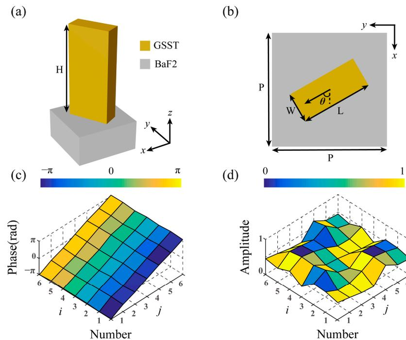
**Figure 2.** Simulated results for the meta atom. (a) Three-dimensional and (b) top view of the meta atom. (c) The simulated transmitted cross-polarized phase shift at A- and C-state. (d) The simulated transmitted cross-polarized amplitude at A- and C-state.  $i$  and  $j$  represent the number of the meta atom while the color of the pixel corresponds to the results at A-state and the position of each pixel indicates the results at C-state.
