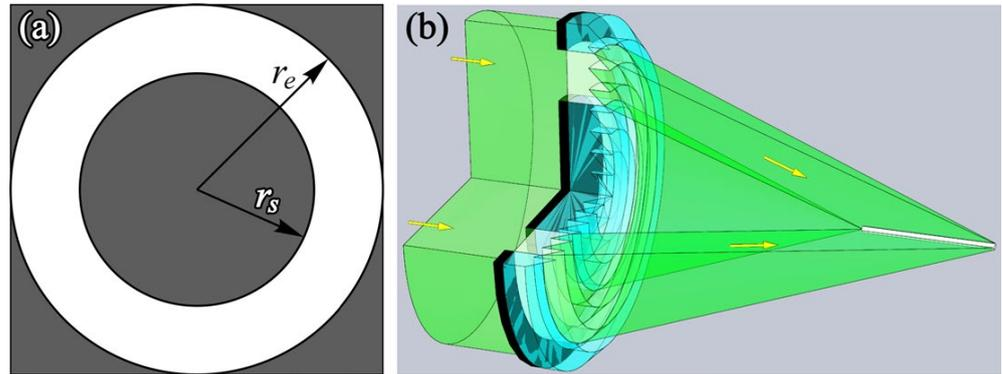
**Figure 1.** (a) View of the annular slot. (b) Geometric-optical illustration of the formation of a light segment on the optical axis.
