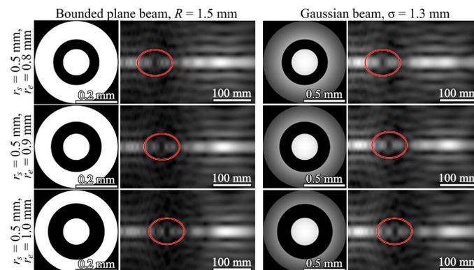
**Figure 6.** Comparative modeling of the optical bottles formation due to radiation blocking by an annular screen under illumination with a bounded flat and the Gaussian beam (the amplitude distribution along the optical axis is shown  $x \in [-0.2$  mm;  $0.2$  mm],  $z \in [50$  mm;  $400$  mm]).
