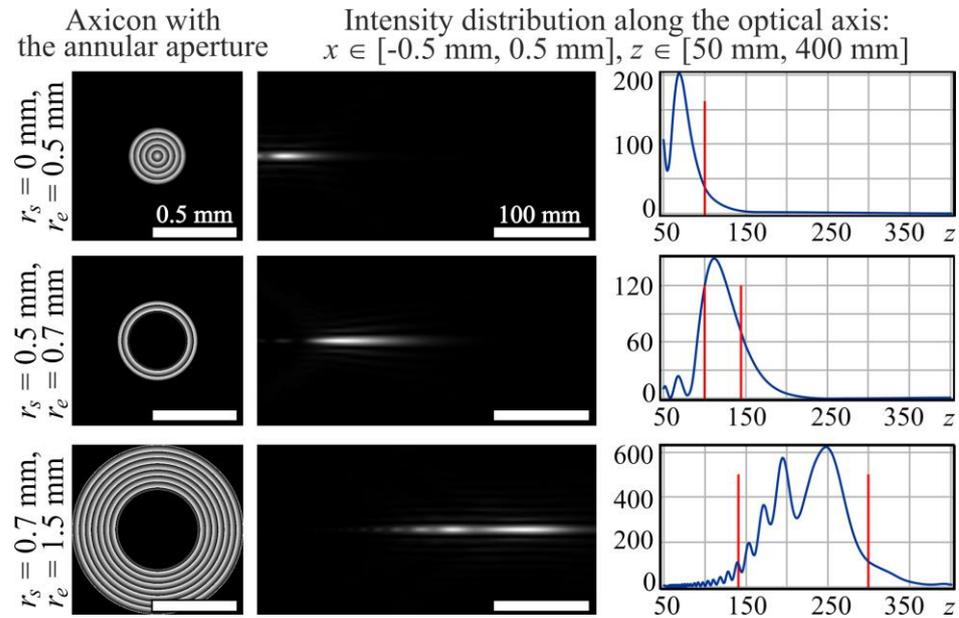
**Figure 2.** Simulation results of the formation of axial light segments with different lengths and positions due to variations in the parameters of the annular aperture were obtained using Equation (2).
