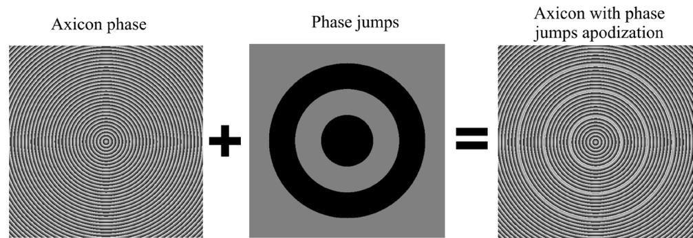
Figure 8. Illustration of axicon apodization by phase jumps ( $\pi$ -shifts between black and grey).
