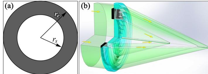
**Figure 3.** Illustration of the formation of an optical bottle due to radiation blocking by an annular screen: (a) view of the annular slot and (b) geometric-optical visualization of the formation of an optical bottle on the optical axis.
