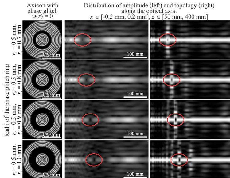
**Figure 7.** Modeling results for the formation of optical bottles due to axicons with phase apodization  $\psi(r) = 0$  in Equation (21) under Gaussian beam illumination.
