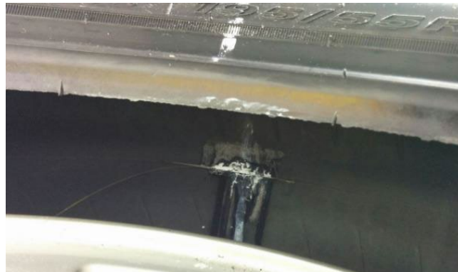
Figure 10. FBG-based strain sensor attached to the inner surface of the tire [44].
