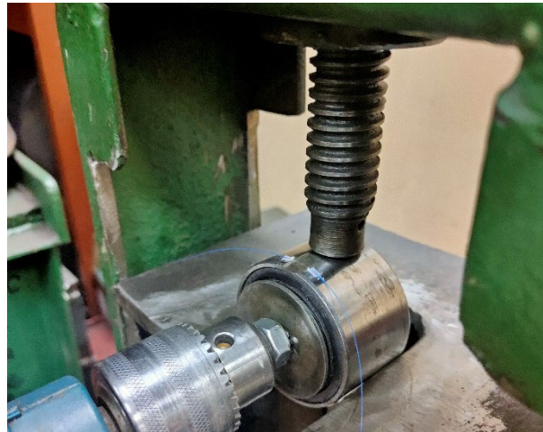
Figure 9. Automotive load-sensing bearing with AFBS sensor during static load testing [13].
