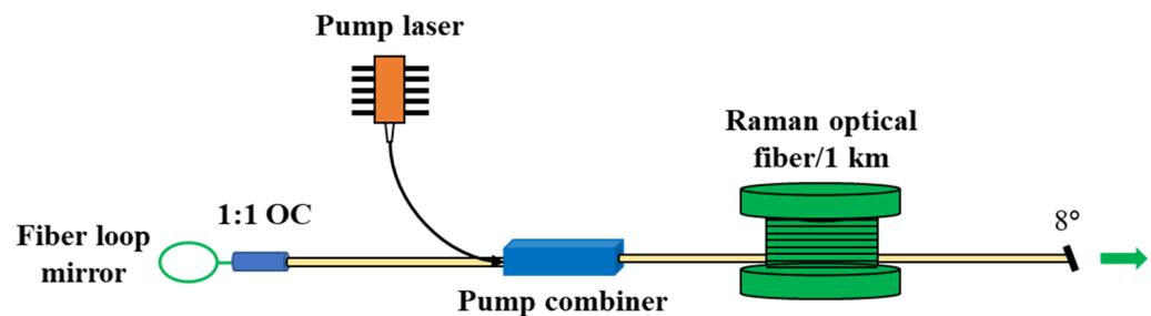
**Figure 1.** Structure of the multi-wavelength random Raman fiber laser.
