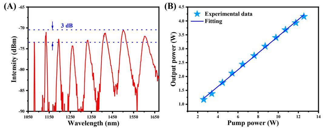
Figure 2. (A) Optical spectrum of the multi-wavelength RRFL; (B) Total output power of the multi-wavelength RRFL.
