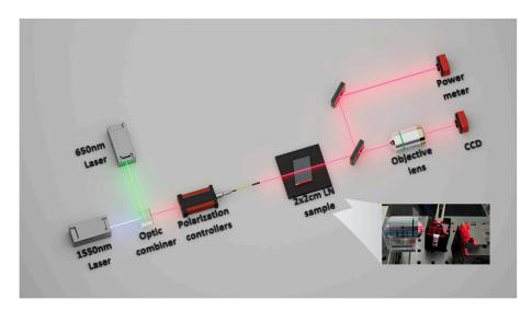
**Figure 6.** The schematic and physical representation of near-field mode measurement are illustrated. We utilize lasers with wavelengths of 1550 nm and 650 nm, which are combined and coupled into a single-mode fiber. The polarized light is then output through a polarization controller, coupled into the LN sample via a bias-preserving fiber, and finally guided through a waveguide. The output is received by sub-CCDs and a power meter. The actual test image is displayed in the lower right corner.
