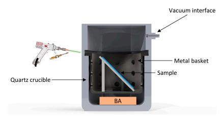
**Figure 1.** VPE vessel. The vessel comprises an inner quartz crucible, a metal carrying basket, and a sample holder. The upper and lower sections are laser-fused, and once the desired pressure is attained, the vacuum interface is heated to create an effective seal through the quartz's collapse.
