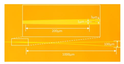
Figure 5. Microscope image of the Y-branch waveguide.
