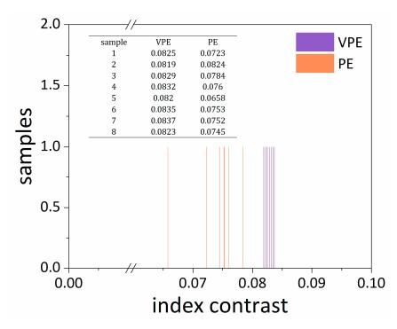
**Figure 3.** Refractive index contrast histograms of VPE and PE samples are presented. To obtain these planar waveguides, two X-cut LN wafers were subjected to VPE at 300 °C for 30 h and PE at 240 °C for 12 h. The VPE waveguide exhibits a very narrow refractive index contrast distribution, in contrast to the PE waveguide, which displays a large refractive index contrast distribution.
