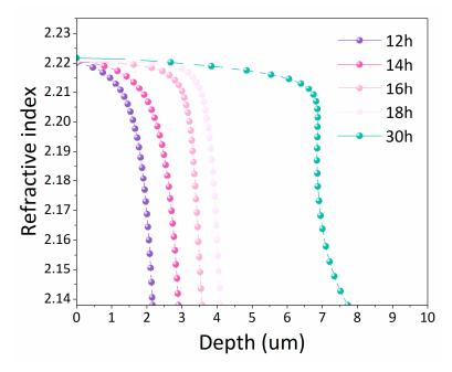
**Figure 2.** Using the IWKB method, we reconstructed refractive index profiles of X-cut LN planar waveguides fabricated via VPE at a wavelength of 1550 nm, employing different reaction times.
