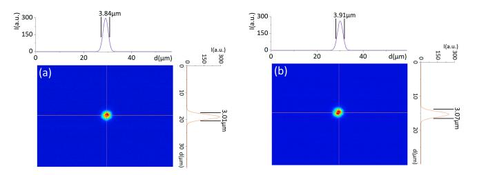
**Figure 7.** Near-field mode images of (**a**) channel waveguide and (**b**) Y-branch waveguide at wavelength 1550 nm.
