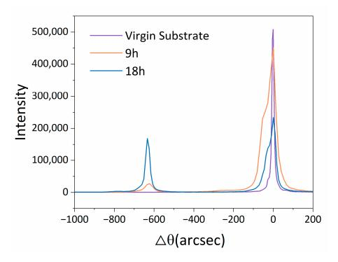
**Figure 4.** X-ray rocking curves were generated through reflections from X-cut VPE planar waveguides (220) subjected to thermal exchange at 300  $^{\circ}$ C for both 9 and 18 h.
