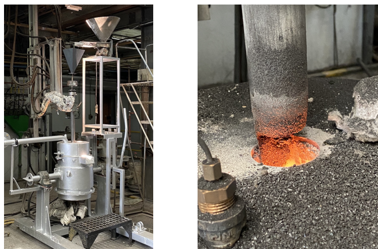
Figure 4. The 100 kVA DC plasma arc furnace pilot facility at Mintek. The furnace vessel is the silver cylinder at lower middle in the left image. A close-up of the electrode extracted from the furnace is shown on the right.
