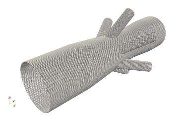
Figure 13. Boundary particles of the discretized geometry for the cylindrical nozzle case.
