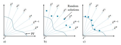
**Figure 1.** Decomposition strategy. (a) A MOP is divided into N sub-problems  $\lambda^1, \ldots, \lambda^N$ ; (b) N random solutions are generated; (c) over a finite number of generations, solutions are simultaneously improved.
