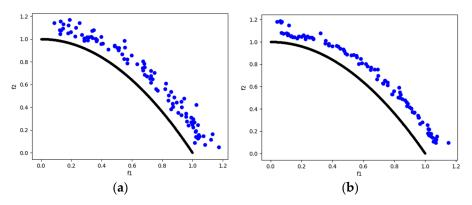
**Figure 12.** The plots of the approximate PFs with the highest HV value against real PF. (a) UF4 approximate PF using MOSA/D-CGO; (b) UF4 approximate PF using MOSA/D-DE.
