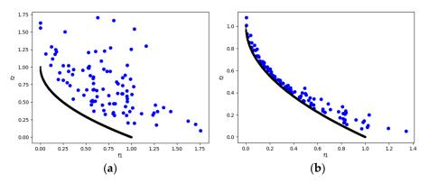
**Figure 10.** The plots of the approximate PFs with the highest HV value against real PF. (a) UF2 approximate PF using MOSA/D-CGO; (b) UF2 approximate PF using MOSA/D-DE.
