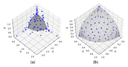
**Figure 4.** The plots of the approximate PFs with the highest HV value against real PF. (a) DTLZ2 approximate PF using MOSA/D-CGO; (b) DTLZ2 approximate PF using MOSA/D-DE.
