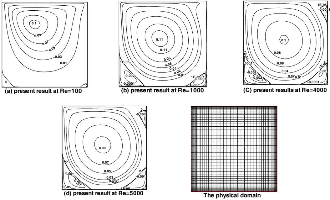
Figure 2: (a-d) Stream function contours and physical domain Clustering grid (51 × 51)
