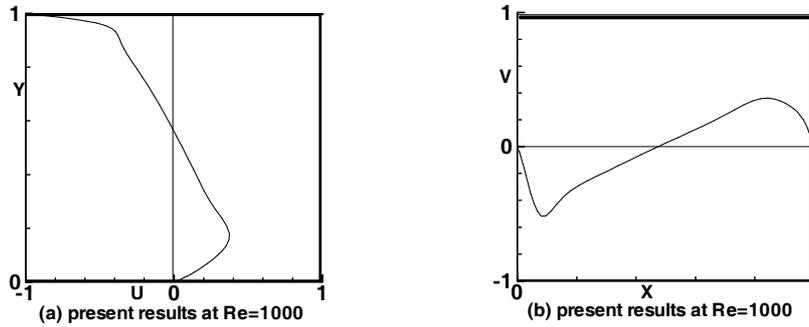
Figure 4: (a) U-Velocity profiles at the centerline of the cavity
