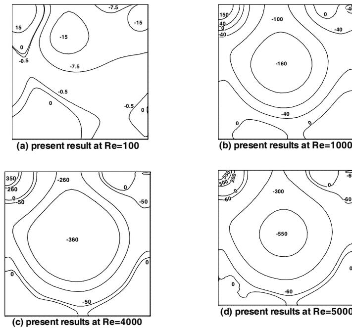
Figure 5: (a-d) Pressure coefficient contours
