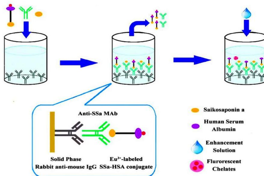
Figure 9. Schematic diagram of the TRFIA system for SSa detection [128].
