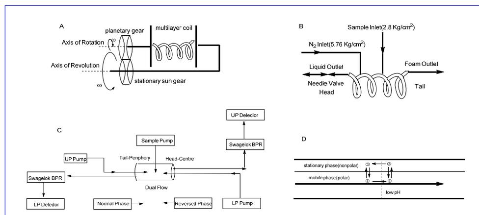
**Figure 4.** Schematic diagram of different types of HSCCC [47]. (A) The synchronous planetary motion of a multilayer coil separation column; (B) design of the coiled column for dual HSCCC; (C) Design of the coiled column for foam HSCCC; (D) mechanism of pH-zone-refining HSCCC.
