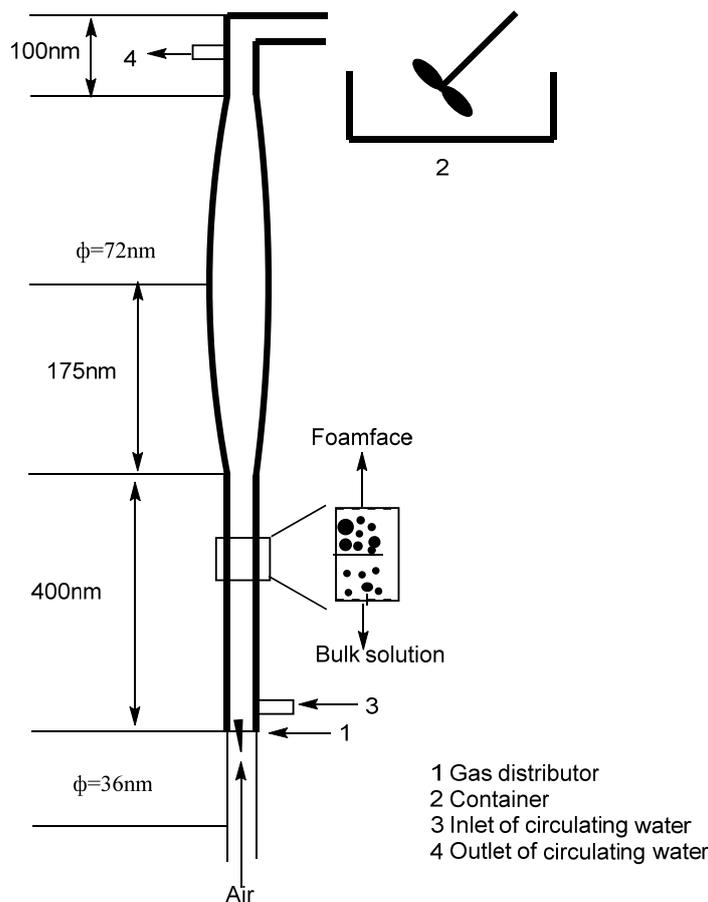
Figure 5. Experimental apparatus of foam fractionation [48].
