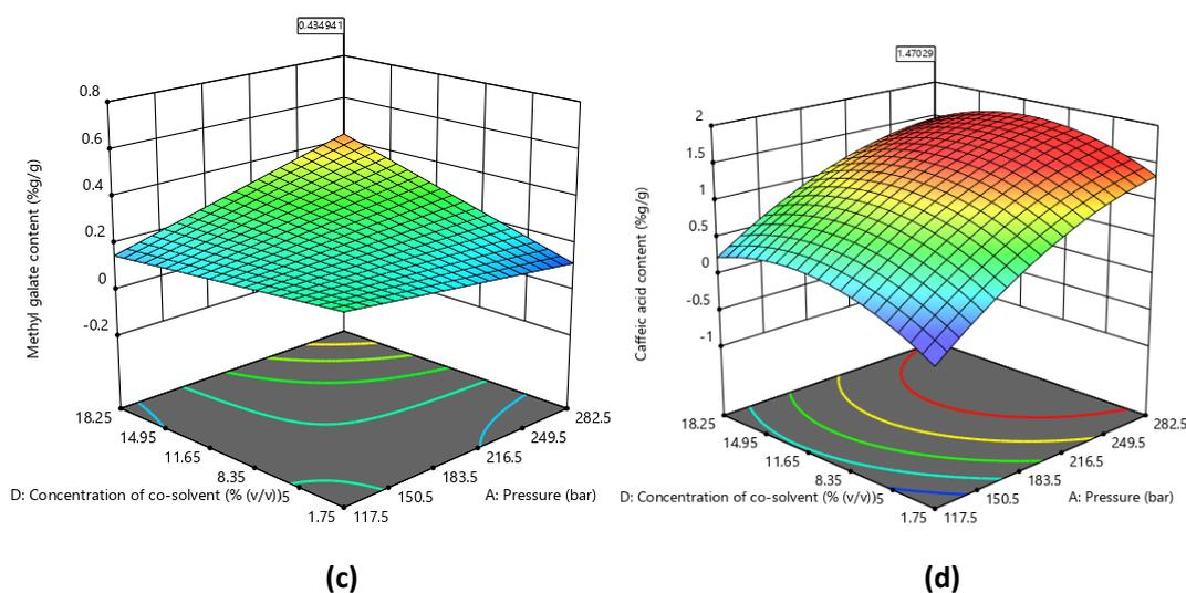
**Figure 3.** Effect of pressure and concentration of co-solvent on (a) extraction yield, (b) gallic acid content, (c) methyl gallate content, and (d) caffeic acid content.
