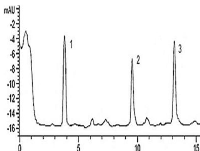
**Figure 7.** HPLC analysis of phenolic compounds extracted using SC-CO<sub>2</sub> with 80% (v/v) ethanol-water as a co-solvent, at 40 °C and 250 bar from leaves of *L. pumila*: (1) gallic acid, (2) methyl gallate, and (3) caffeic acid.
