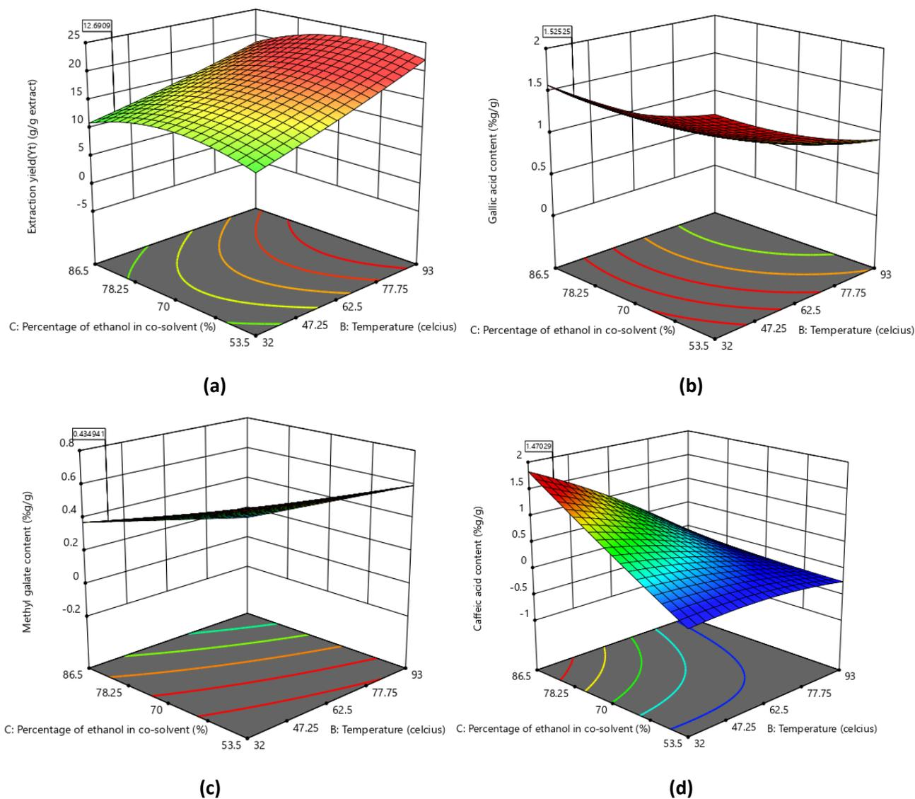
**Figure 4.** Effect of temperature and percentage of ethanol in co-solvent on (a) extraction yield, (b) gallic acid content, (c) methyl galate content, and (d) caffeic acid content.
