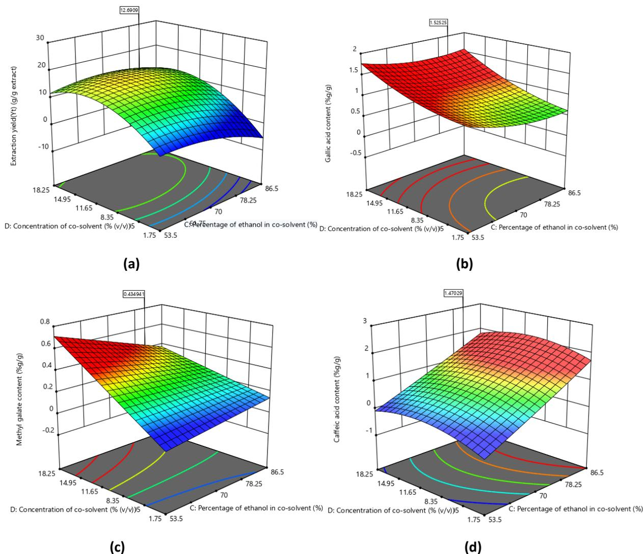
**Figure 6.** Effect of percentage of ethanol in co-solvent and co-solvent concentration on (a) extraction yield, (b) gallic acid content, (c) methyl gallate content, and (d) caffeic acid content.
