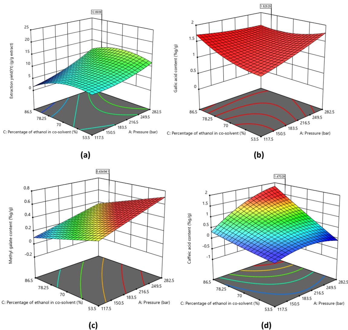
**Figure 2.** Effect of pressure and percentage of ethanol in co-solvent on (a) extraction yield, (b) gallic acid content, (c) methyl galate content, and (d) caffeic acid content.
