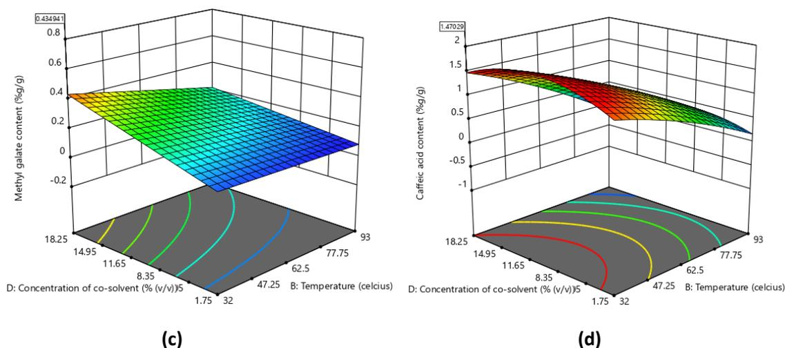
**Figure 5.** Effect of temperature and concentration of co-solvent on (a) extraction yield, (b) gallic acid content, (c) methyl gallate content, and (d) caffeic acid content.
