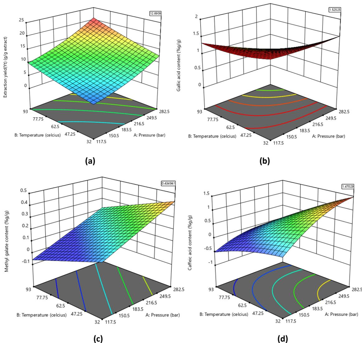
**Figure 1.** Effect of pressure and temperature on (a) extraction yield, (b) gallic acid content, (c) methyl galate content, and (d) caffeic acid content.
