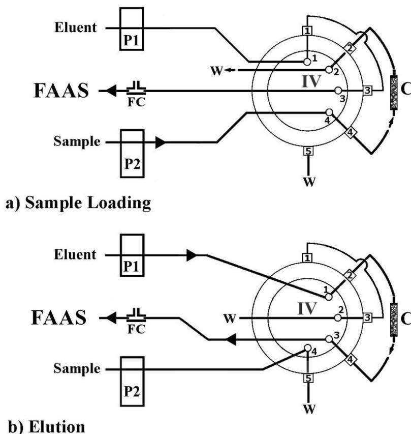
**Figure 2.** Schematic representation and operation sequences of FI-FAAS (a) step 1, sample loading and (b) step 2, elution (Table 1), IV; injection valve, P1 and P2; peristaltic pumps, W; waste, C; microcolumn, FC; flow compensation unit.
