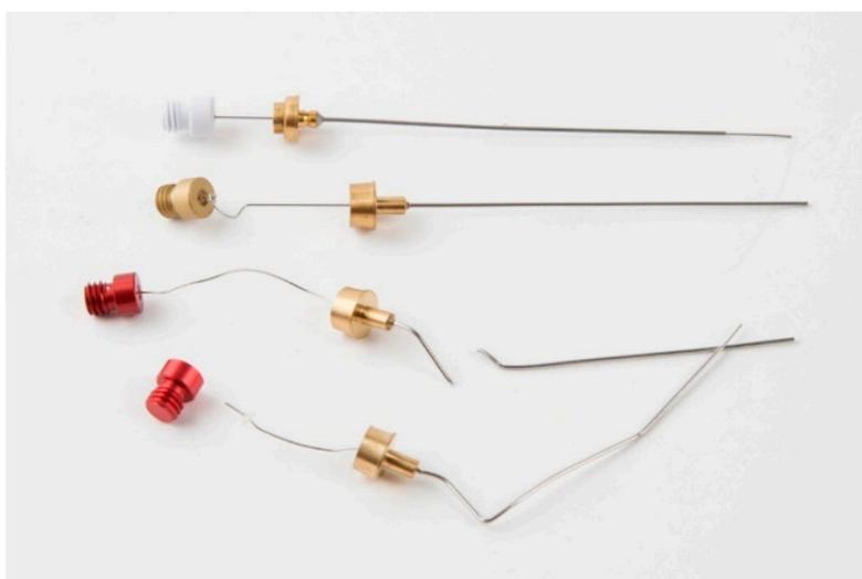
**Figure 4.** Mechanical failures common to traditional SPME fibers.
