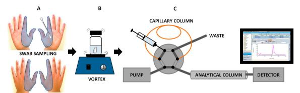
**Figure 1.** Schematic diagram of the steps for DPA analysis: (**A**) web and palm of the hand sampling (zone sampling in blue), (**B**) vortex-assisted extraction, and (**C**) IT-SPME-capillary liquid chromatography (CapLC) system.
