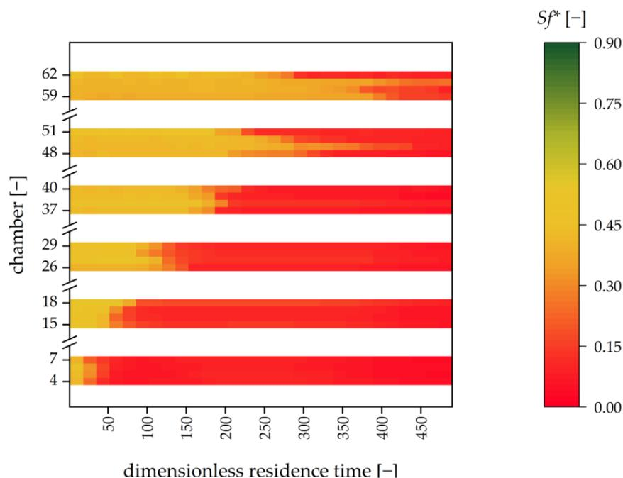
**Figure 4.** Retention values over time for the 6 viewing windows (containing 4 chamber–duct combinations each) of a transparent single-disc rotor. White areas indicate intransparent regions of the rotor. Phase system used: Arizona N, mobile phase flow:  $15 \text{ mL}\cdot\text{min}^{-1}$ ,  $22 \text{ }^\circ\text{C}$ , 750 rpm, tripled runs.
