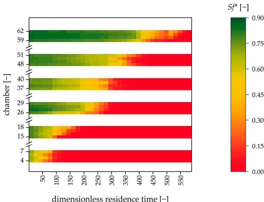
**Figure 5.** Retention values over time for the 6 viewing windows (containing 4 chamber–duct combinations each) of a transparent single-disc rotor. White areas indicate intrtransparent regions of the rotor. Phase system used: Arizona U, mobile phase flow: 15 mL·min<sup>-1</sup>, 22 °C, 750 rpm, tripled runs.
