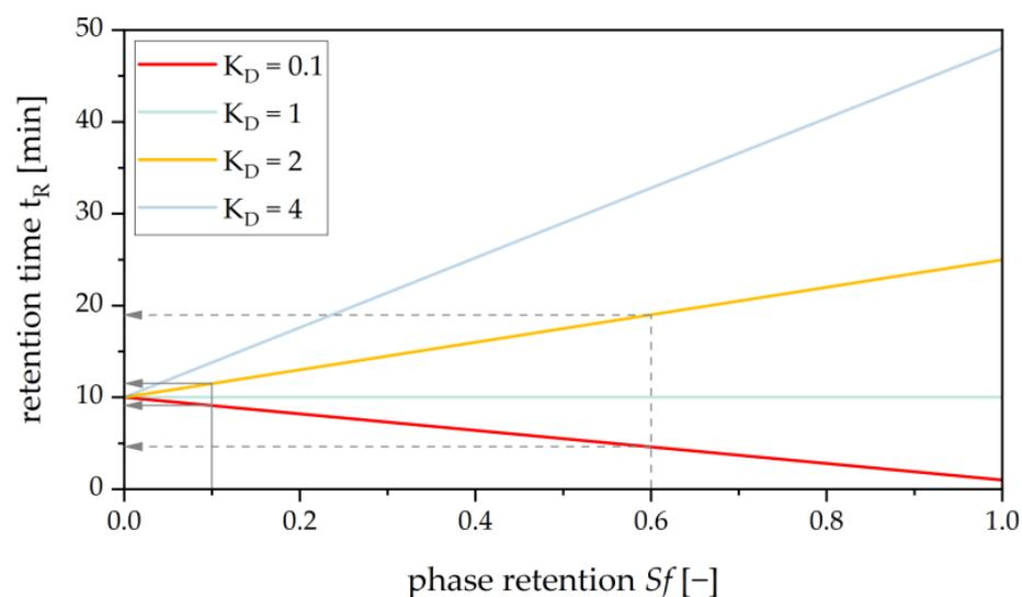
**Figure 1.** Retention time over proportion of stationary phase/retention ( $Sf$ ) inside a CPC apparatus for different  $K_D$  values.
