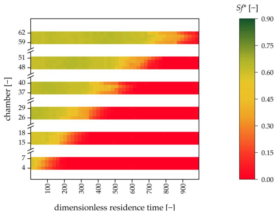
**Figure 6.** Retention values over time for the 6 viewing windows (containing 4 chamber–duct combinations each) of a transparent single-disc rotor. White areas indicate intransparent regions of the rotor. Phase system used: Arizona G, mobile phase flow:  $20 \text{ mL}\cdot\text{min}^{-1}$ ,  $22 \text{ }^\circ\text{C}$ , 750 rpm, tripled runs, hydrodynamic residence time: 0.46 min.
