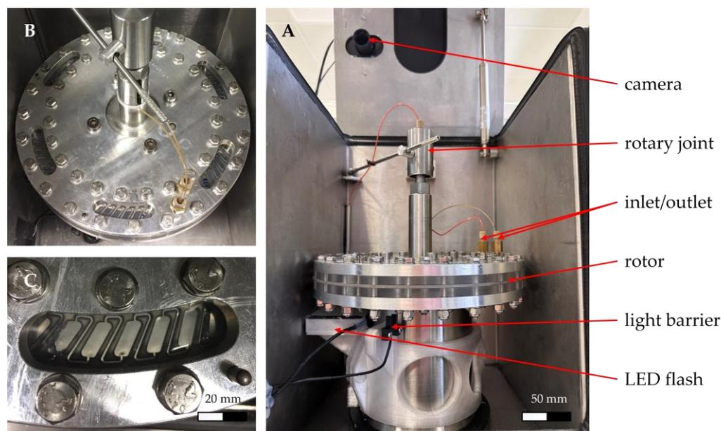
**Figure 2.** (A) CPC assembly: The rotor is flanged to an electric motor with an upright rotation axis. Two rotary joints (the lower one not shown) ensure fluid flow from the inlet to the outlet. The light barrier is triggered once per revolution, whereby an LED flash and a camera are actuated. (B) Top view of the rotor with six viewing windows. (C) The first viewing window with four chambers and interconnecting ducts is completely visible.
