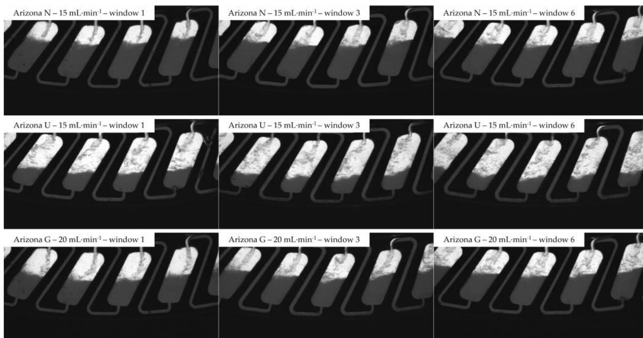
**Figure 3.** Hydrodynamics with a constant flow regime for different phase systems after 10 dimensionless hydrodynamic residence times. Phase system used: Arizona N, U, and G, 22 °C, FCPC single-disc rotor, desc. mode, 750 rpm.
