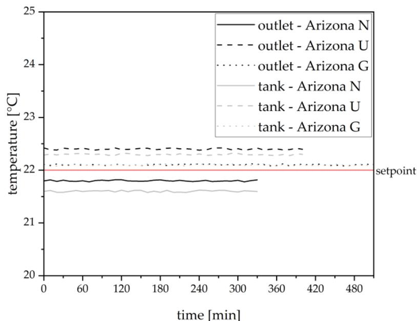
**Figure 7.** Temperature measurements of the mobile phase directly at the outlet of the apparatus and in the mobile phase storage tank (tempered) for different phase systems. The red line indicates the setpoint for the corresponding water bath.
