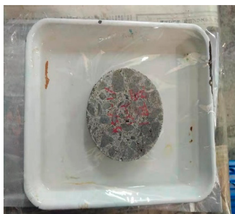
Figure 2. The setup of water absorption test.
