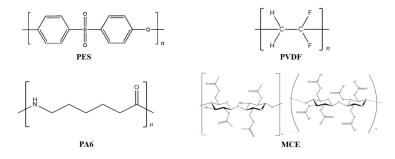
Figure 2. The molecular structures of PES, PVDF, PA6 and MCE.
