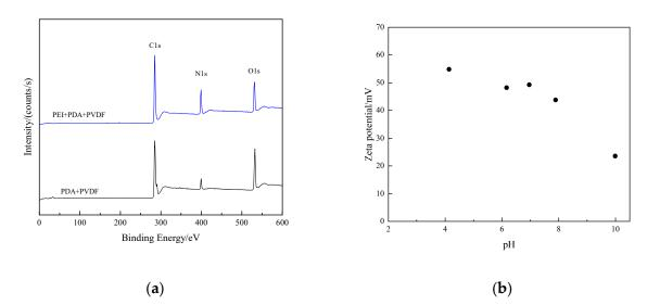
Figure 9. (a) XPS wide scans and (b) Zeta potential of MA.
