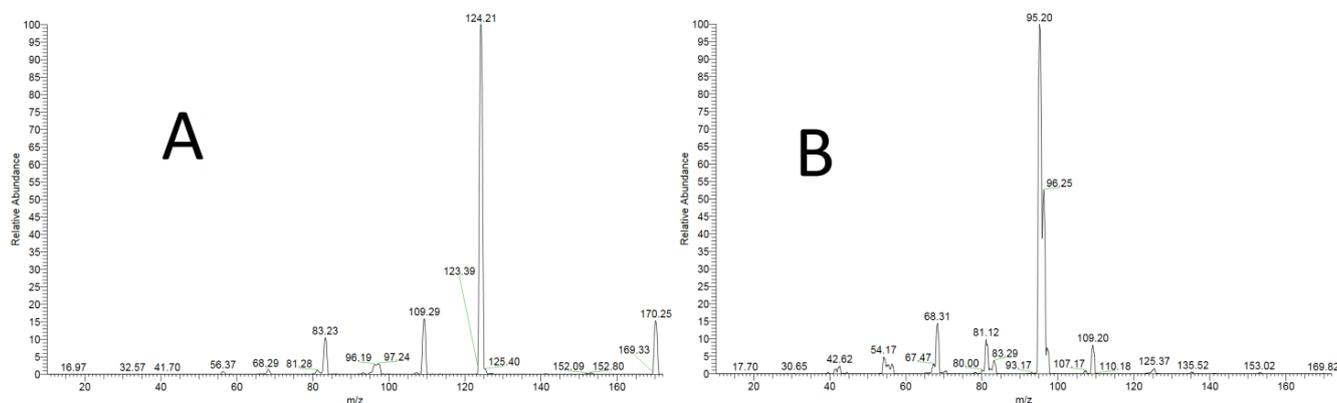
**Figure 2.** (A): Mass spectrum at a CE of 15 V for  $\tau$ -MH. The spectrum is an average of 50 scans, from 10 to 172  $m/z$  for the precursor 170  $m/z$ . Ion 124 is the most intense peak in the spectrum, (B): Mass spectrum at a CE of 30 V for  $\pi$ -MH. The spectrum corresponds to the average of 50 scans, from 10 to 172  $m/z$  for the precursor 170  $m/z$ . Ion 95 is the most intense peak in the spectrum. Readers should refer to Figure S4 for more details.
