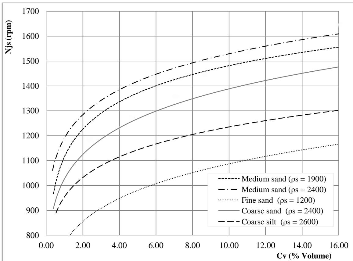
Figure 7. Effect of particle density on  $N_{js}$ .
