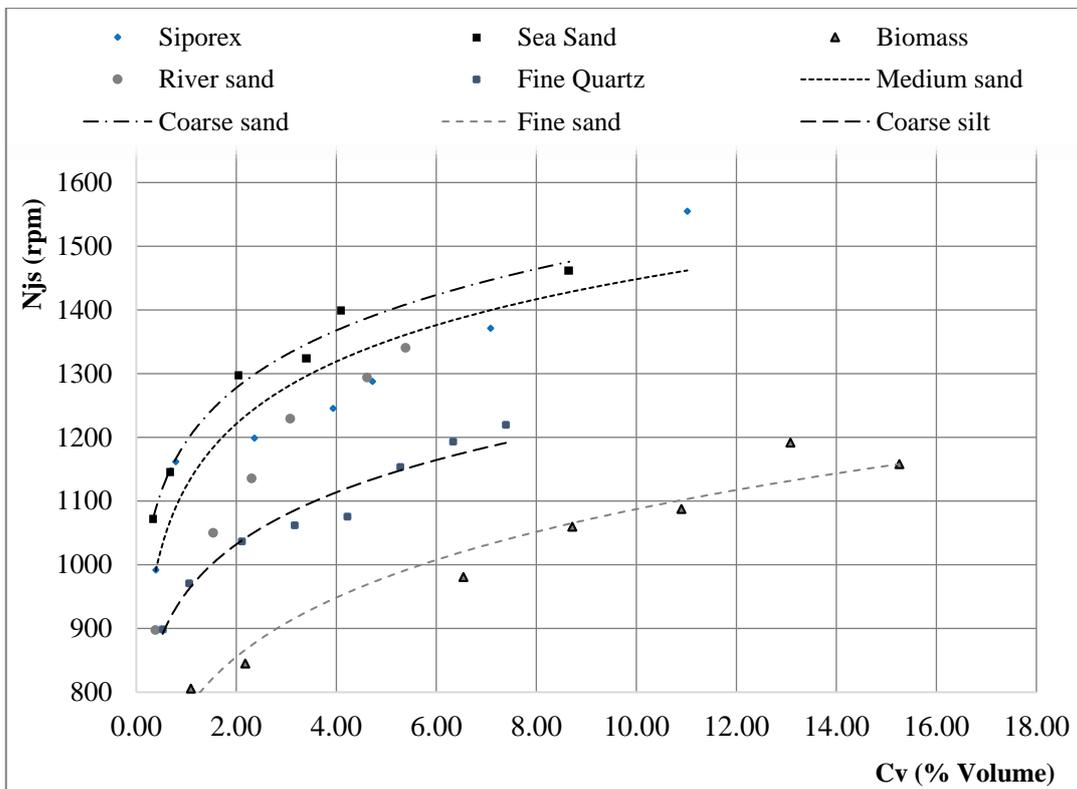
Figure 6. Effect of particle concentration on  $N_{js}$ .
