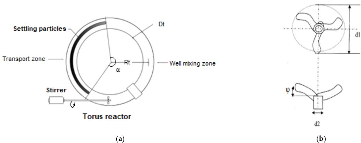
Figure 1. Torus reactor (a) description of settling bed (b). The marine screw impeller [2].
