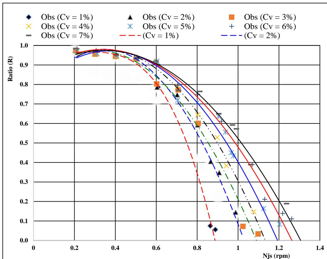
Figure 2. Example of determination of  $N_{js}$  by extrapolation.
