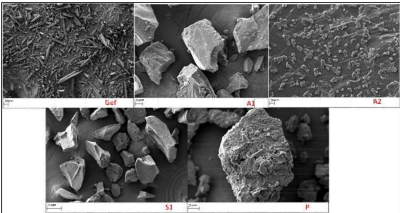
**Figure 4.** SEM images of pure Gef and various SDs (A1-MW, A2-MW, S2-MW, and P-MW) prepared using microwave method.
