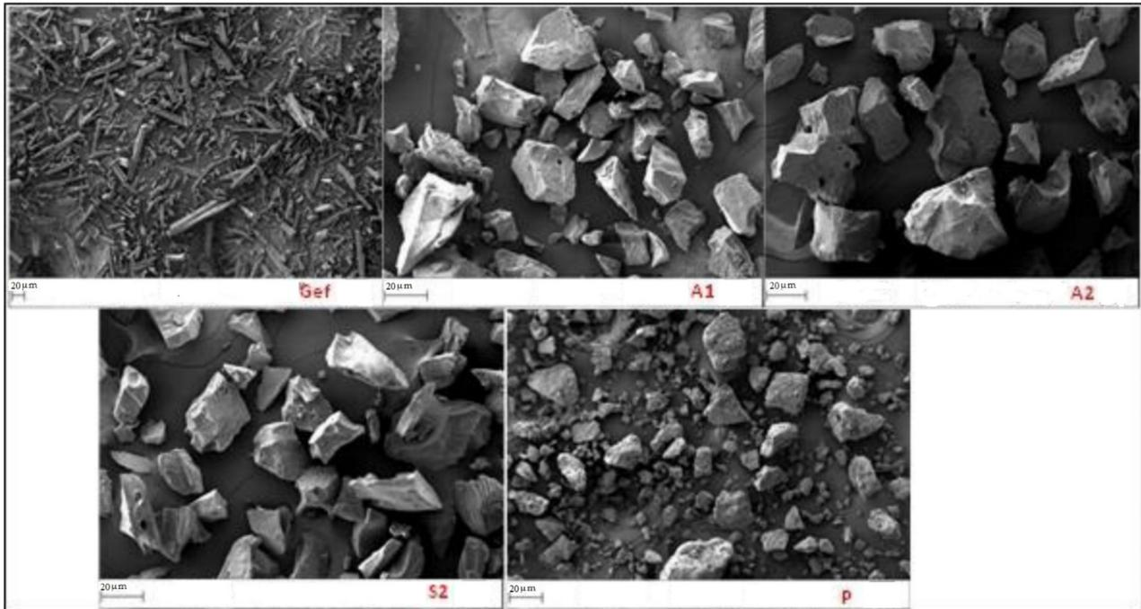
**Figure 3.** Scanning electron microscope (SEM) images of pure Gefitinib (Gef) and various SDs (A1-F, A2-F, S2-F, and P-F) prepared using fusion method.
