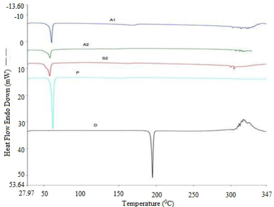
**Figure 1.** Differential scanning calorimetry (DSC) thermograms for pure drug (D) and various SDs prepared using fusion method.
