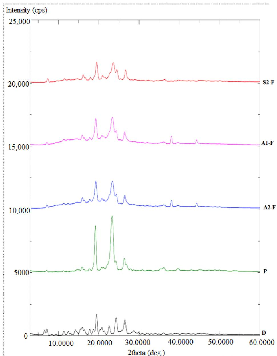
**Figure 7.** Powder X-ray diffraction (PXRD) spectra for pure Gef and different Gef-SDs formulations prepared using fusion method.
