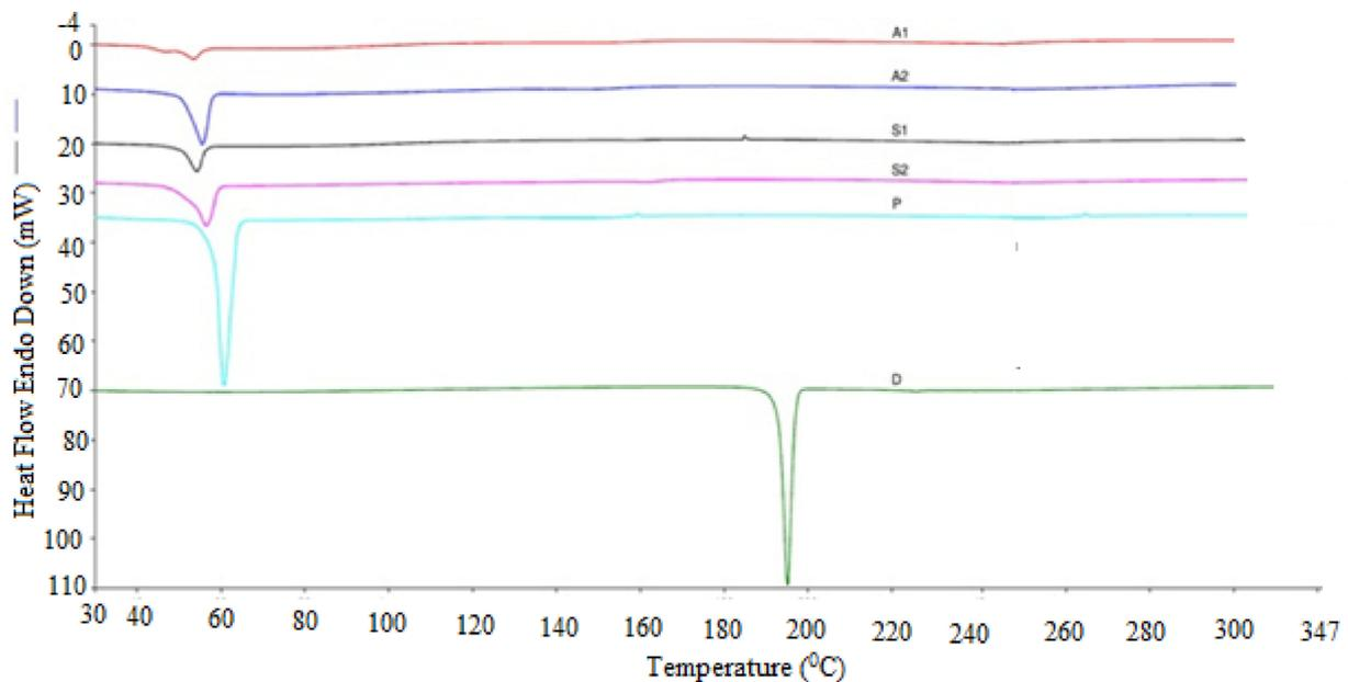
**Figure 2.** DSC thermograms for pure drug (D) and various SDs prepared using microwave method.
