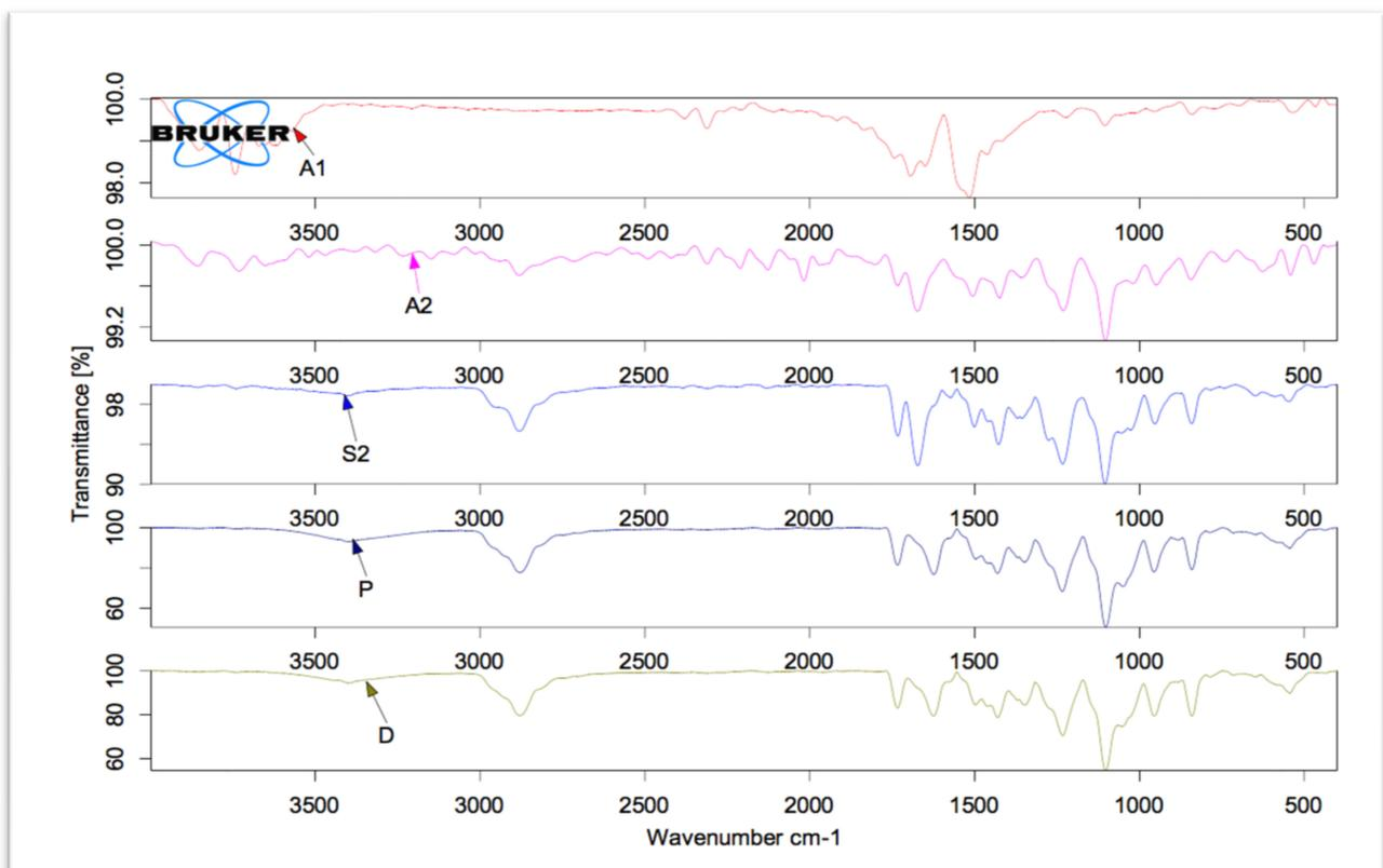
**Figure 5.** Fourier transforms intra-red (FTIR) spectra for pure Gef and different Gef-SDs formulations prepared using fusion method.
