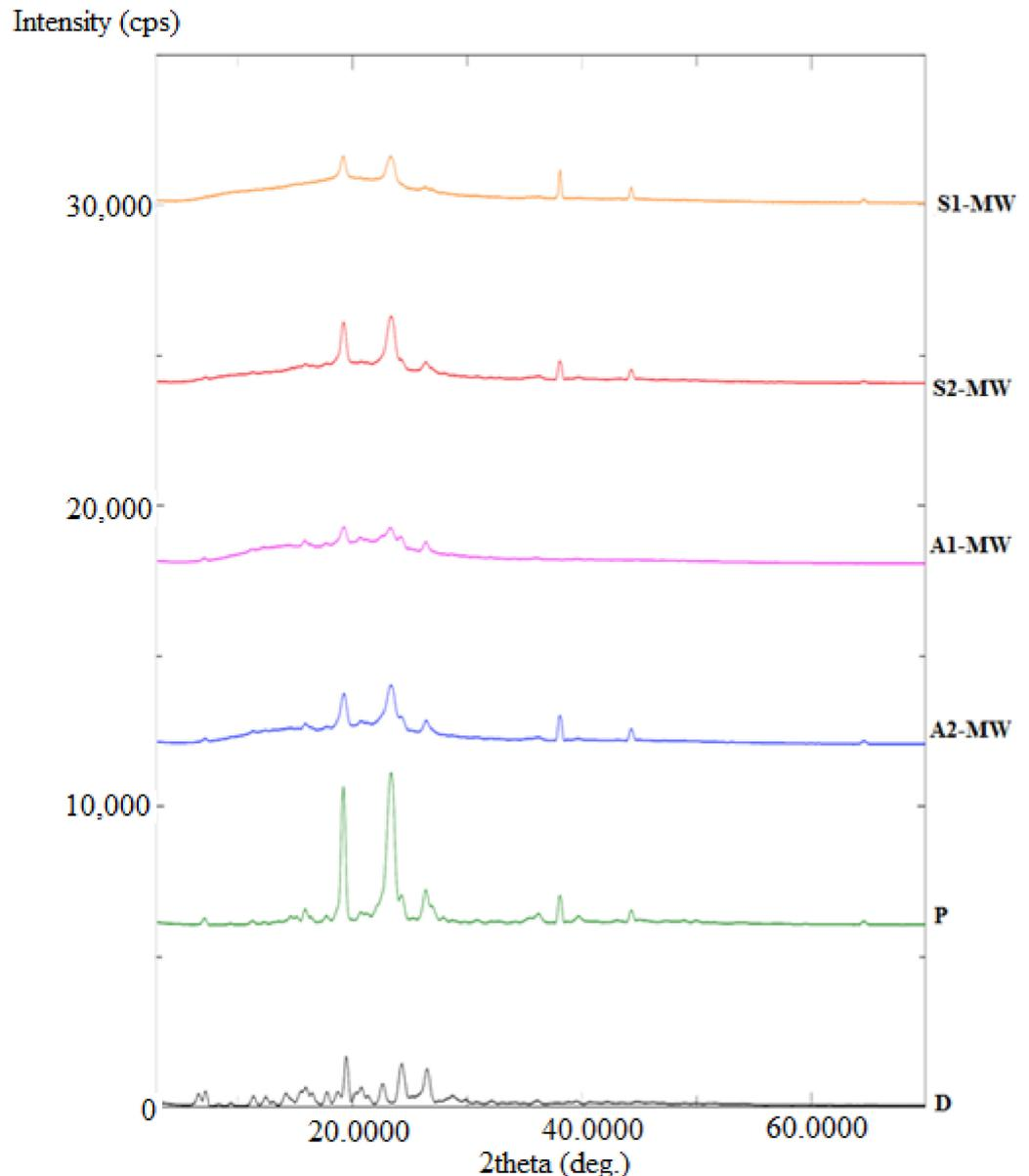
**Figure 8.** PXRD spectra for pure Gef and different Gef-SDs formulations prepared using microwave method.
