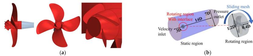
**Figure 8.** Geometrical configuration of the simulation for the POW test: (a) the geometry of the propeller with PBCF and (b) numerical towing tank with boundary conditions.
