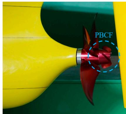
Figure 1. PBCF installed at propeller hub [6].
