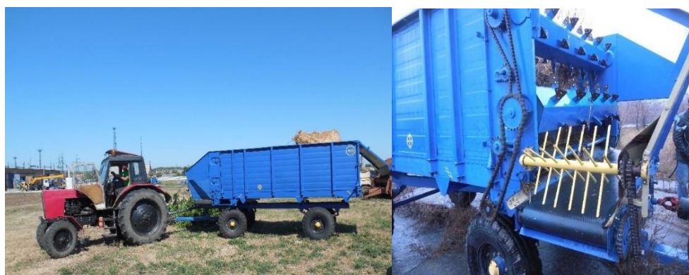
Figure 1. General view of equipment for the technological process of making straw bedding with rotary finger working bodies (for clarity and complete display of the drive and the working body, the protective barriers were dismantled at the time of photo-fixation).
