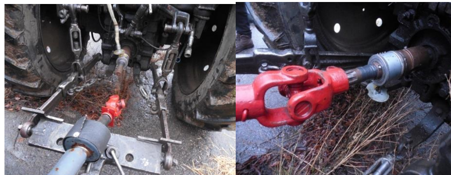
Figure 3. Determination of torque on the selection shaft tractor power.
