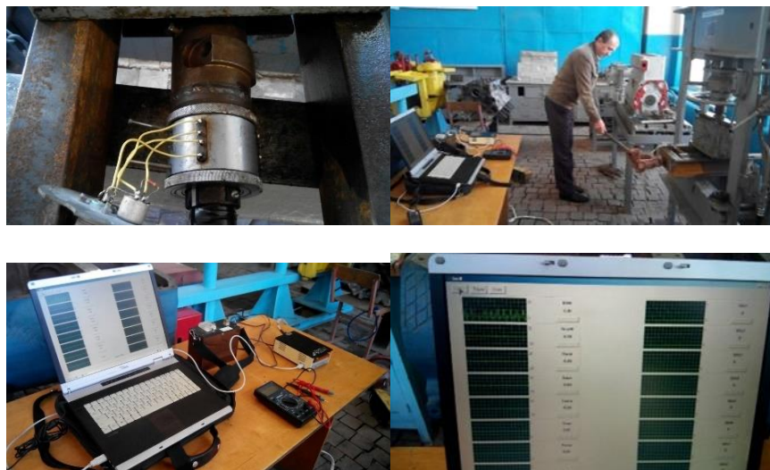
Figure 5. Calibration of mercury amalgamated current collector.
