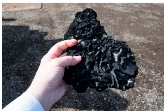
Figure 4. Photograph of crust from top of biofuel slurry after evaporative cooling of reactor.
