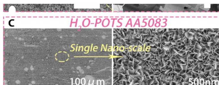
Figure 5. SEM images of aluminum substrates after immersion in boiling water and hydrophobization. Reproduced with permission from [24].
