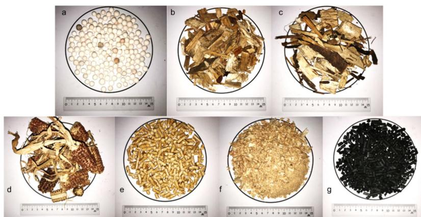
**Figure 2.** Deployed feedstocks (a) alumina oxide spheres, (b) wood chips, (c) residues from forestry, (d) corn cobs, (e) wood pellets, (f) saw dust and (g) biochar.
