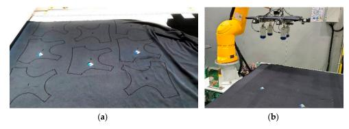
Figure 13. Automatic cutting process: (a) preparation for cutting; (b) transfer of cut fabrics for robot gripping.
