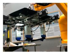
**Figure 19.** Photographs of the robot-based gripping system sequential operations of moving to, grasping, and transferring the target fabric object.
