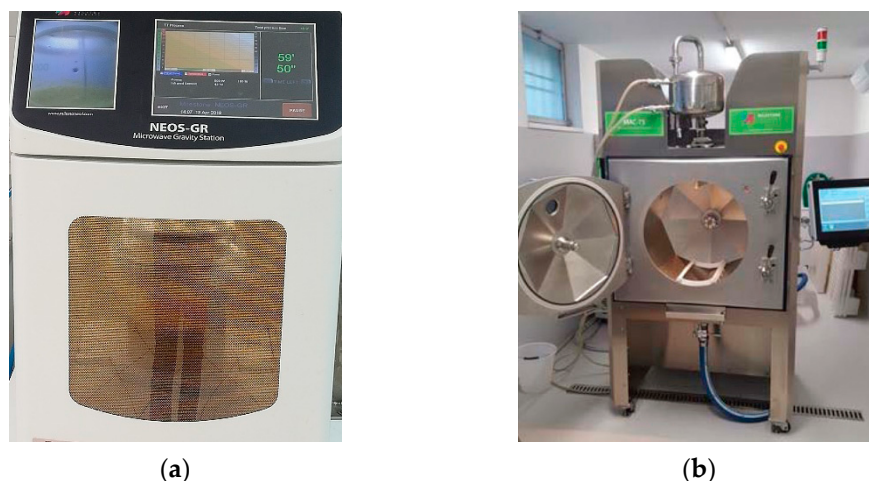
Figure 4. (a) Lab scale and (b) industrial scale of microwave-assisted extractors.
