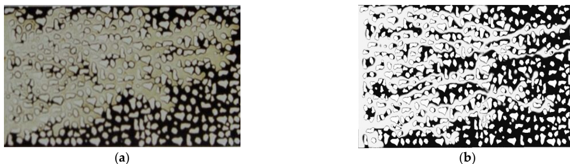
Figure 6. Flow distribution within the micromodel at rupture time. Injection velocity: 10 ft/day and IFT 0.03 mN/m. (a) Experimental and (b) simulation.
