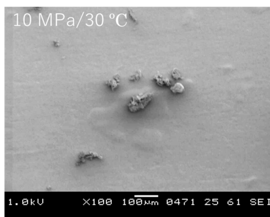
Figure 4. Morphology of Lf loaded shellac microparticles produced at different P and T conditions of supercritical CO 2 in the PGSS process.
