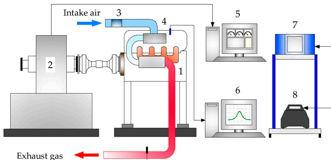
**Figure 1.** Schematic diagram of the experiment set up [43]. 1. Test engine, 2. eddy current dynamometer, 3. air mass sensor, 4. pressure sensor, 5. dynamometer controller, 6. data acquisition system, 7. AVL gas analyzer, 8. smoke opacity meter.
