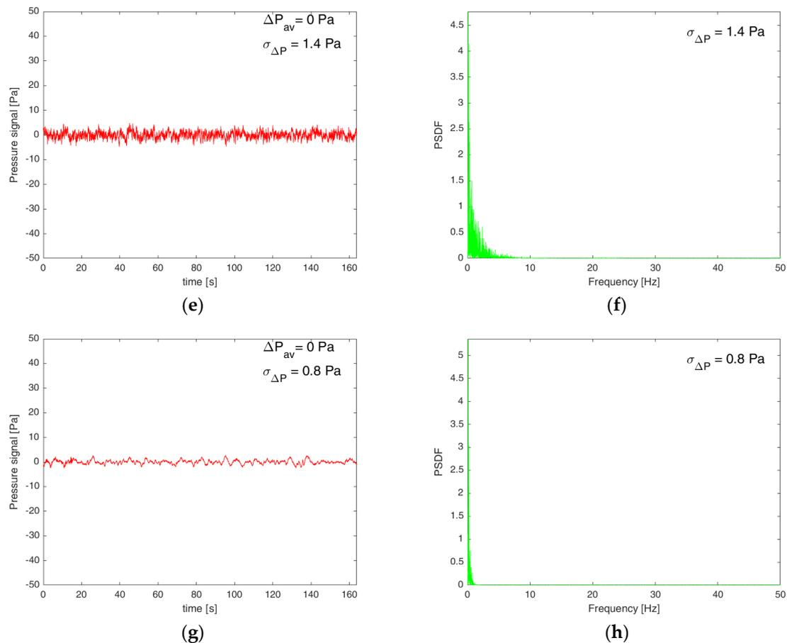
**Figure 9.** Pressure fluctuation signals from the fluidized bed made of ILM and ash from WSP with related PSDF (power spectral density functions), at  $u = 2u_{mf}$  of ilmenite: (a,b) at 750 °C, (c,d) at 850 °C, (e,f) at 900 °C, and (g,h) at 1000 °C.
