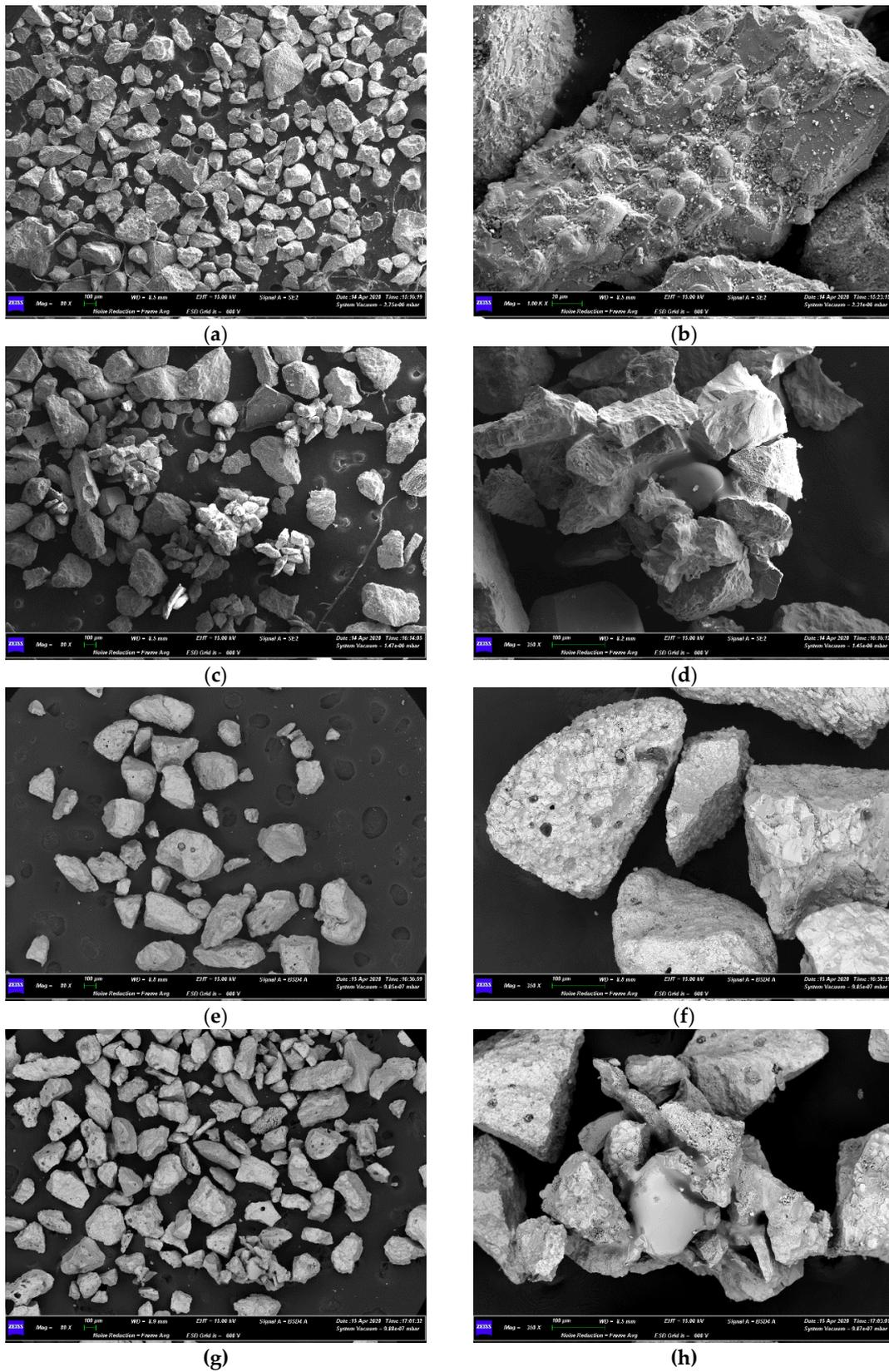
**Figure 14.** SEM micrographs of SIB after fluidization steps: with WSP ash after the step at 700 °C at 80× (a) and 1000× (b), with WSP ash after the step at 1000 °C at 80× (c) and 350× (d), with WSP-T3 ash after the step at 700 °C at 80× (e) and 350× (f), and with WSP-T3 ash after the step at 1000 °C at 80× (g) and 1000× (h).
