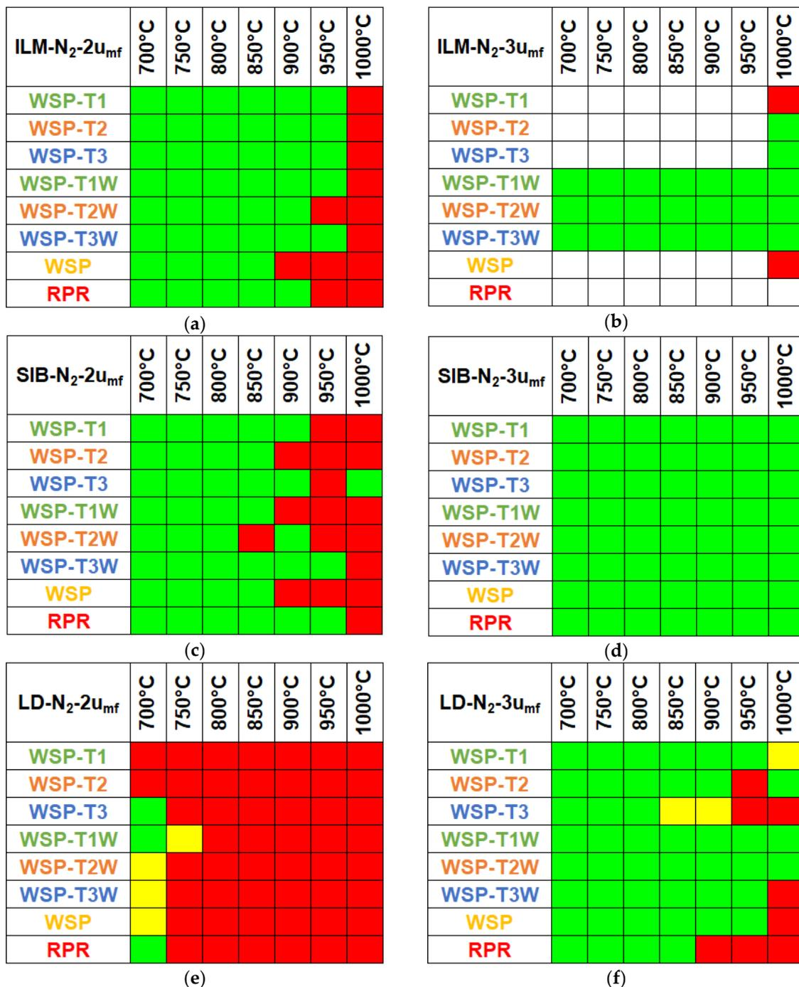
**Figure 10.** Evaluation of fluidization quality based on the experimental PSDFs. Legend: green square = bubbling bed (corresponding to the situation described by Figure 9a–d), yellow square = bubbling fluidization fading out (corresponding to the situation described by Figure 9e,f), red square = no bubbling (corresponding to the situation described by Figure 9g,h), and white = not acquired.
