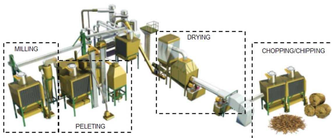
**Figure 1.** Scheme of the solid biofuels pretreatment unit at biorefinery and bioenergy centre (BIO2C).
