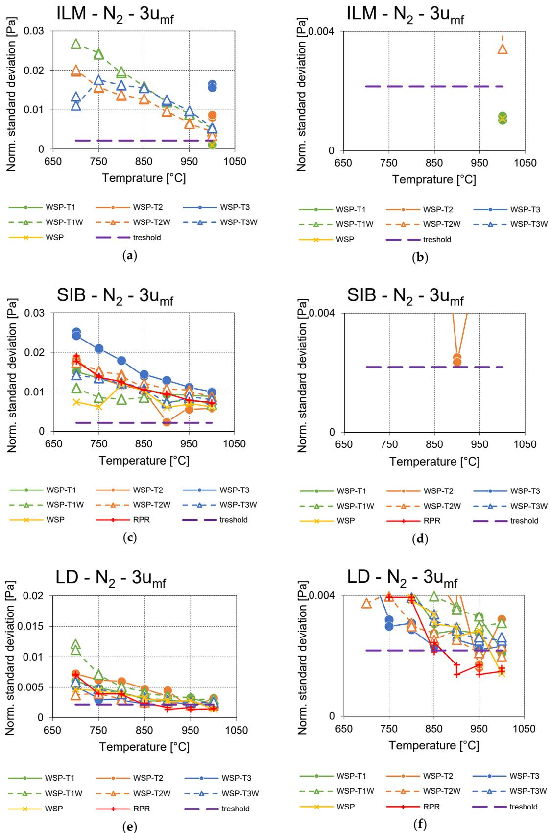
**Figure 12.** Normalized experimental standard deviations as functions of temperature during fluidization of OCs–ash couples at nominal 3 u<sub>mf</sub> (a,c,e), with respective magnifications (b,d,f).
