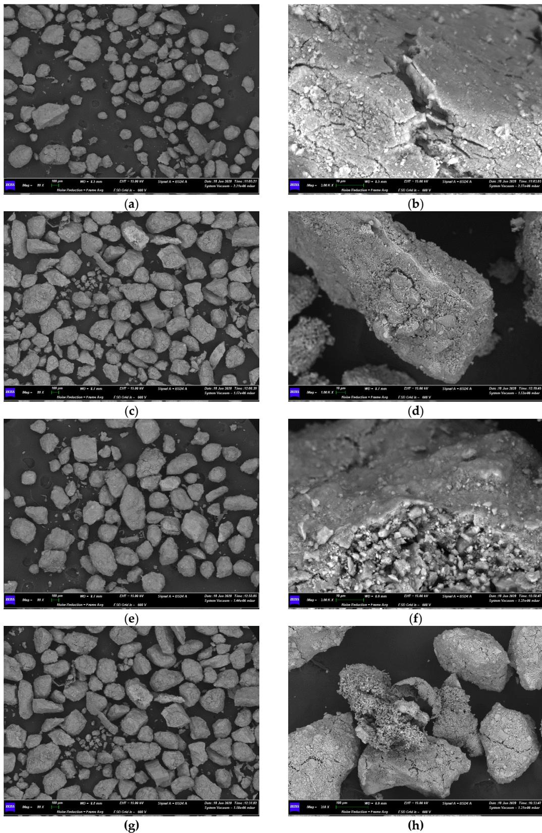
**Figure 15.** SEM micrographs of LD after fluidization steps: with WSP ash after the step at 700 °C at 80× (a) and 3000× (b), with WSP ash after the step at 1000 °C at 80× (c) and 1000× (d), with WSP-T3 ash after the step at 700 °C at 80× (e) and 3000× (f), and with WSP-T3 ash after the step at 1000 °C at 80× (g) and 350× (h).
