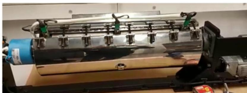
**Figure 2.** Torrefaction laboratory rotating batch reactor.
