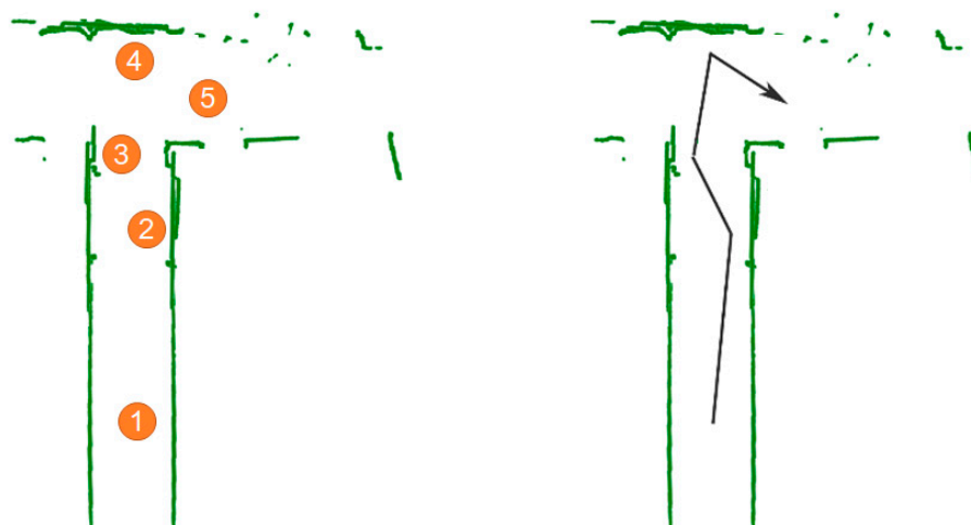
Figure 29. Integrated image of scanned result in third autonomous scanning experiment. The numbers indicating the positions after movement from the starting position of the autonomous scanner ( left ); also, the trajectory of the autonomous scanner is indicated ( right ).
