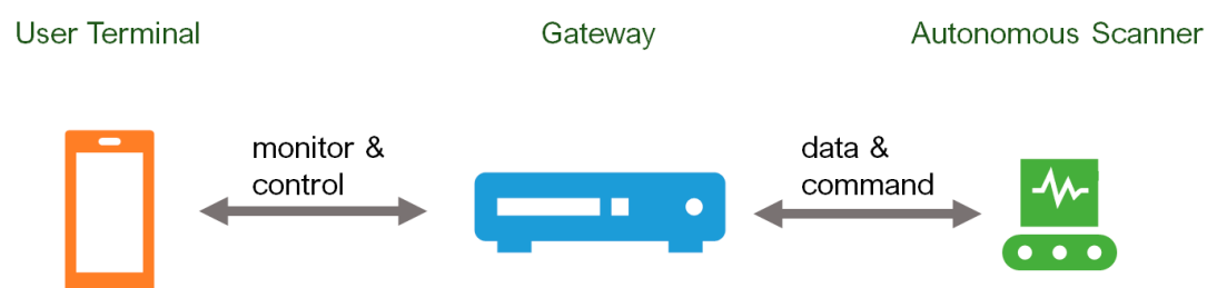
Figure 1. Conceptual architecture of proposed autonomous scanning system. It is composed of three main parts: a user terminal, a gateway, and an autonomous scanner.
