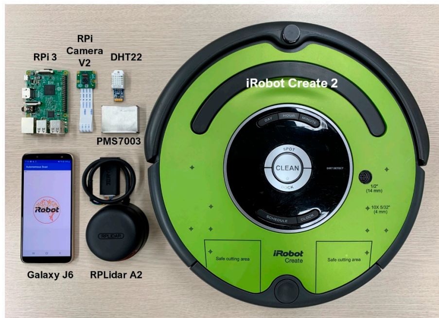
Figure 2. Components of proposed autonomous scanning system. We utilized prototyping platforms such as Raspberry Pi and iRobot Create 2.
