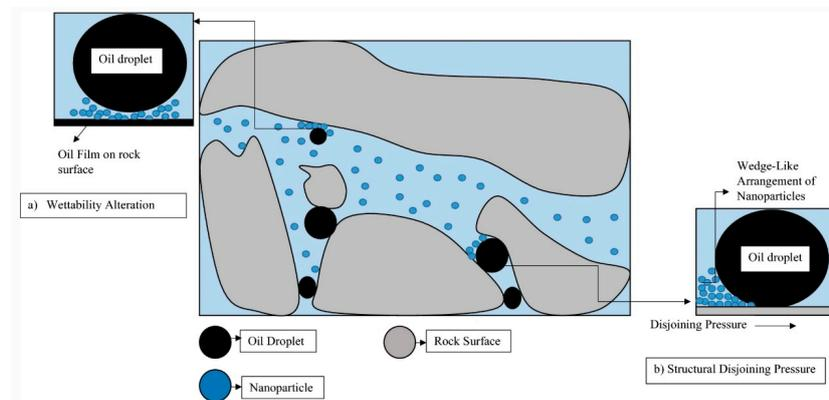
**Figure 2.** Mechanism of NPs EOR. (a) Changing wettability and (b) structural pressure by NPs [31].
