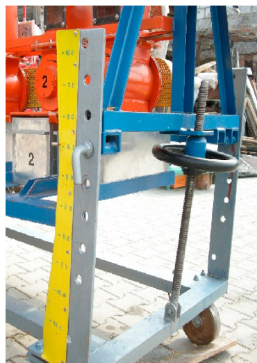
Figure 2. Indicator and control mechanism of the sieve unit inclination angle.
