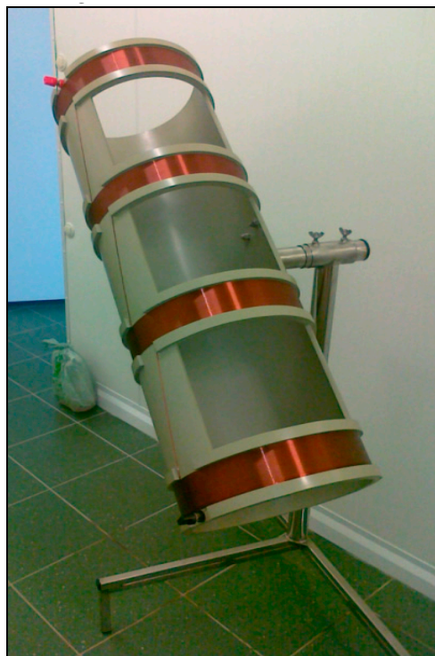
Figure 2. Coil designed for fruit storage at near null GMF (geomagnetic field).
