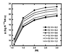
**Figure 7.** Variations in flow function with pressure ratio (PR) and S/H (K/H = 4, D/H = 4).
