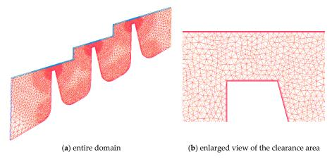
**Figure 3.** Example of the computational domain and meshes (S/H = 0.4).
