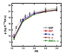
**Figure 5.** Comparison of turbulence models (S/H = 1.0, K/H = 4, D/H = 4).
