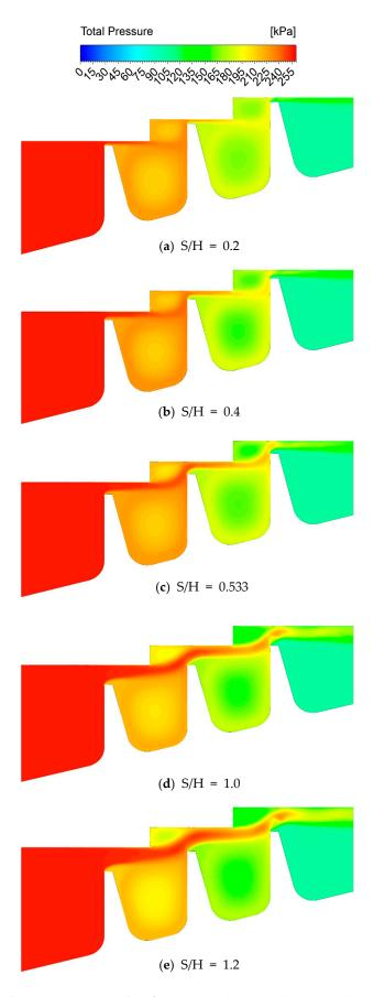
**Figure 9.** Total pressure contour plots for various S/H ratios (PR = 2.5, K/H = 4, D/H = 4).
