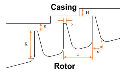
Figure 2. Seal geometry and parameters.
