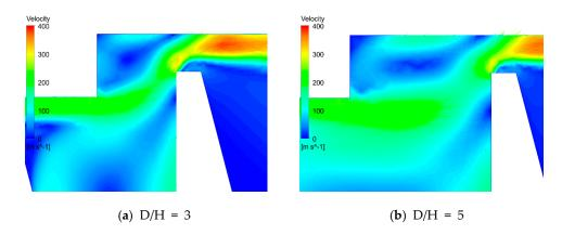
Figure 18. Velocity contour plots for the smallest and largest D/H ratios (PR = 2.5, S/H = 0.6, K/H = 4).
