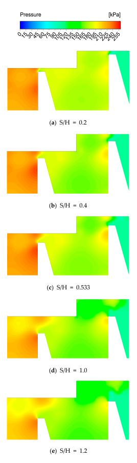
**Figure 10.** Static pressure contour plots for various S/H ratios (PR = 2.5, K/H = 4, D/H = 4).
