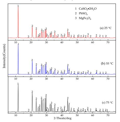
Figure 3. X-ray diffraction patterns of leach residues at different leach temperatures.
