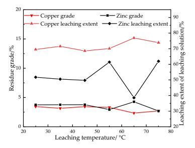
Figure 2. Results of leaching temperature tests.
