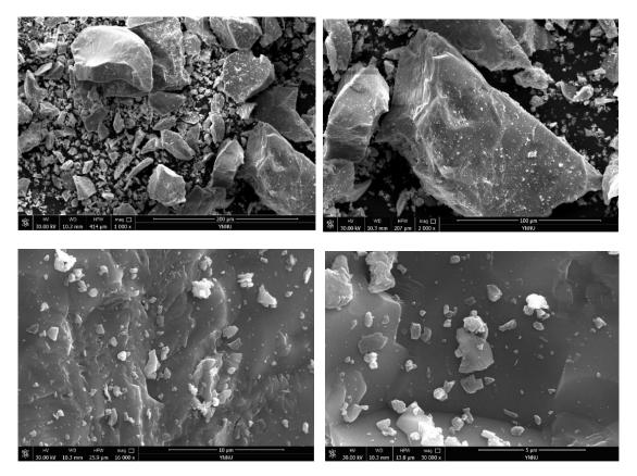
Figure 10. Scanning electron micrograph of morphology of roast calcine (before leaching).
