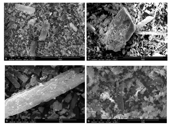
Figure 11. Scanning electron micrograph of morphology of roast calcine (after leaching).
