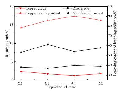
Figure 6. Results of leaching liquid:solid ratio tests.
