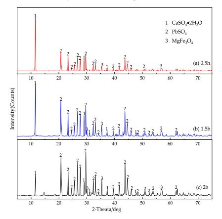
Figure 9. X-ray diffraction patterns of leach residues obtained for different leaching times.
