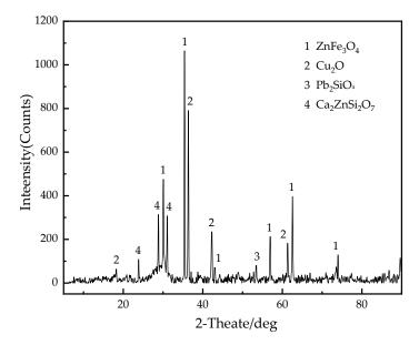
Figure 1. X-ray diffraction pattern of roast calcine.
