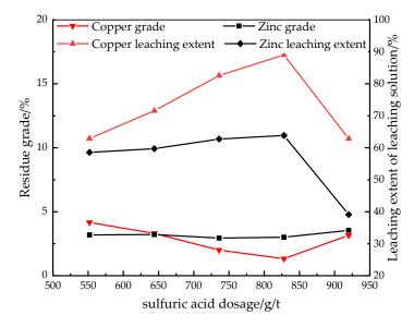
Figure 4. Results of leaching at different sulfuric acid dosage.
