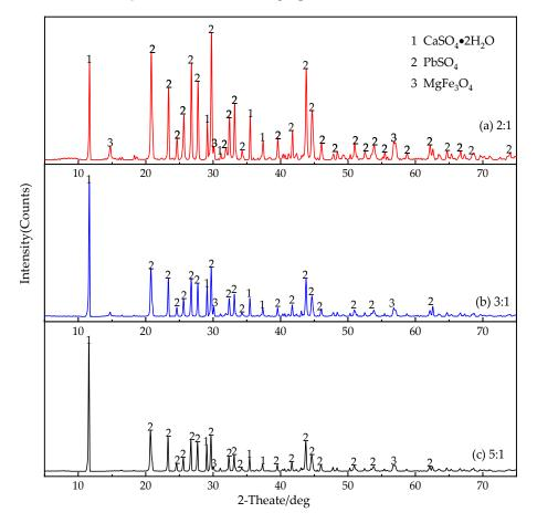
Figure 7. X-ray diffraction patterns of leach residue obtained at different liquid:solid ratios.
