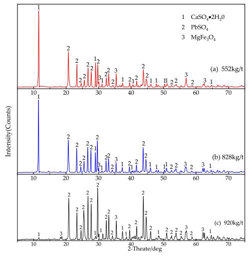
Figure 5. X-ray diffraction patterns of leach residues after leaching at different sulfuric acid dosages.
