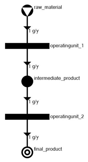
Figure 4. Graphical representation of materials in P-graph.
