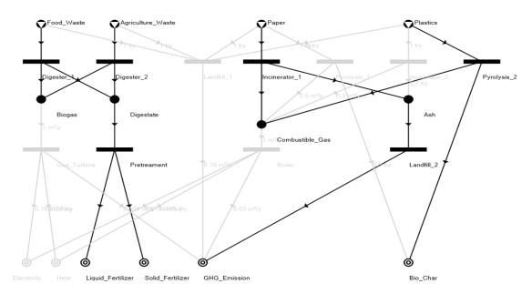
**Figure 9.** Feasible structure with the least environmental impact.
