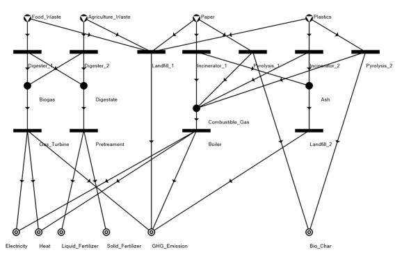
**Figure 5.** A P-graph representation of the municipal solid waste process network.
