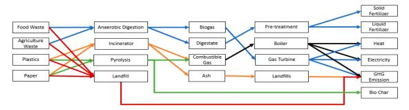
Figure 3. Superstructure for process flow managing MSW in this case study.
