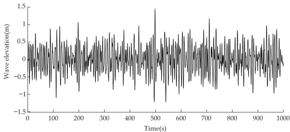
**Figure 12.** The time history of the wave elevation.
