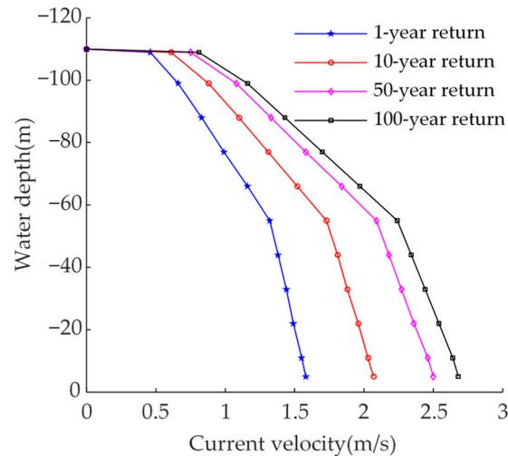
**Figure 11.** The variation of the current velocity at different water depths.
