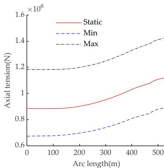
**Figure 16.** Comparison of axial tension forces.
