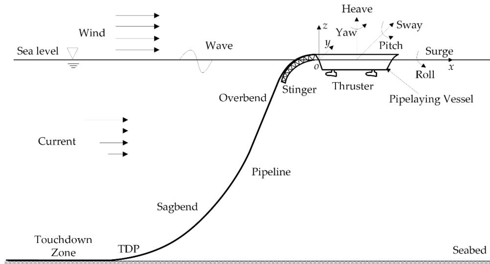
**Figure 1.** Schematic diagram of S-laying pipeline installation.
