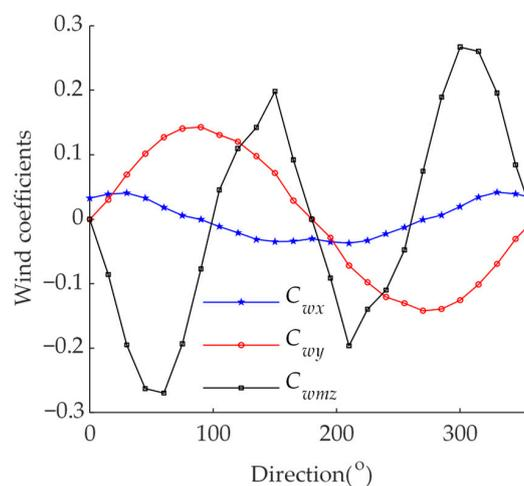
Figure 5. The wind coefficients for HYSY201.
