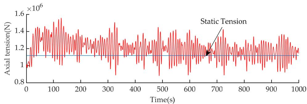
**Figure 15.** Time histories for the pipeline top tension force.
