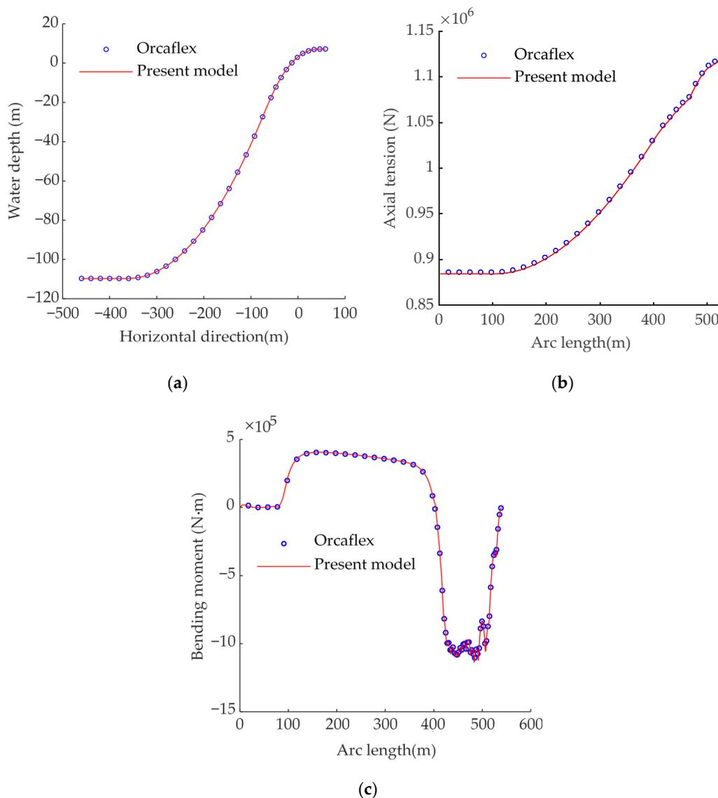
**Figure 10.** Comparison between the present model results and OrcaFlex simulations: (a) configurations; (b) tension forces; and (c) bending moments.
