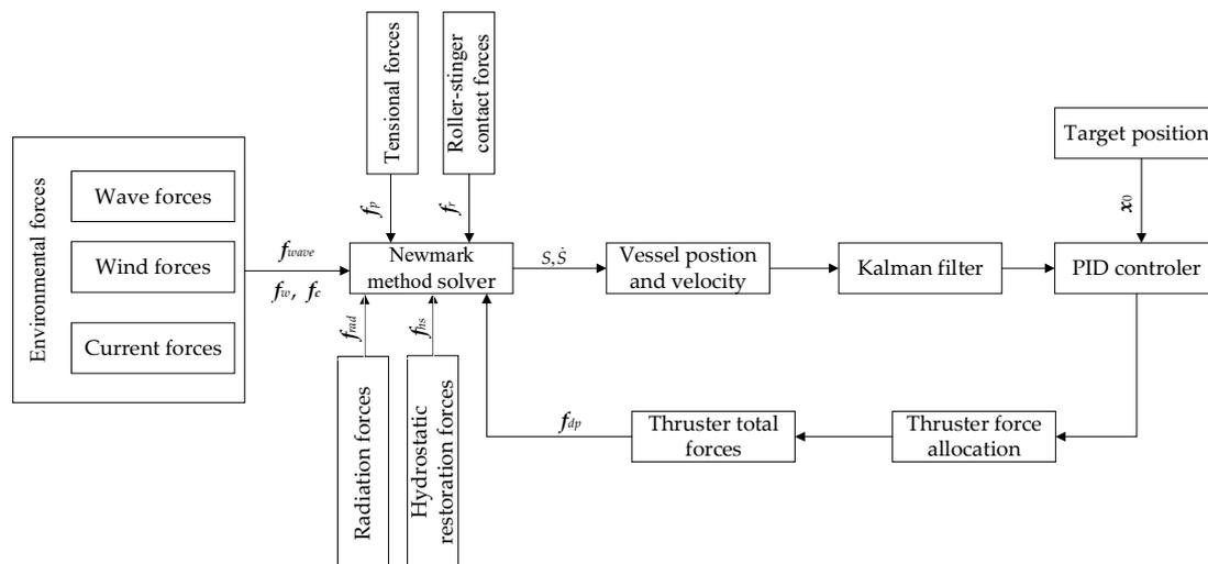
Figure 9. Solution procedure for the coupled model.
