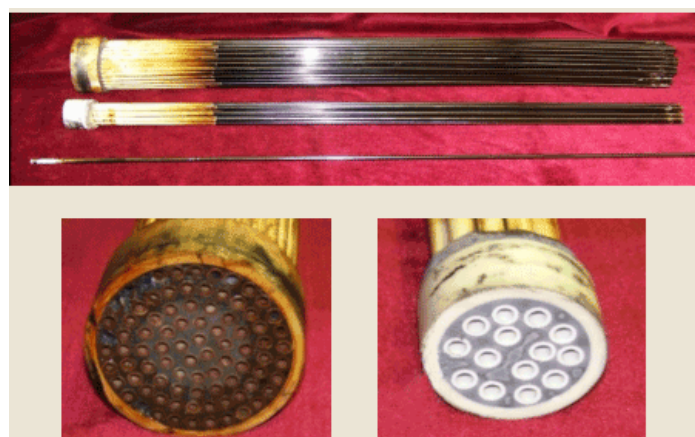
Figure 6. Alumina-supported CMSM tube pilot scale bundle and full-scale bundle produced by MPT. Reproduced with permission from [90], Elsevier, 2014.
