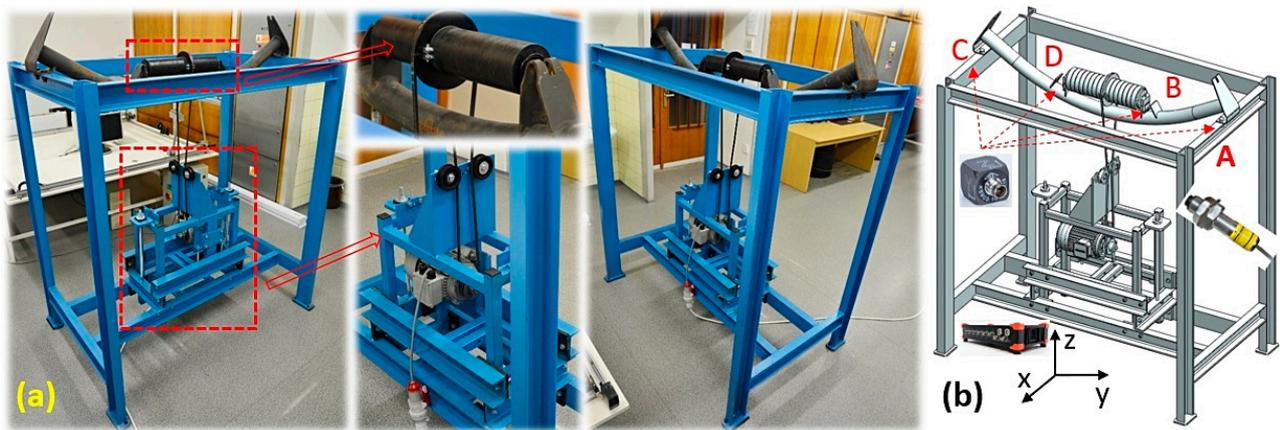
**Figure 16.** (a) Laboratory equipment used to measure the vibration of conveyor rollers, (b) the placement of accelerometers in measuring points B and D on the fixed conveyor idler and in points A and C on the frame on the laboratory equipment.
