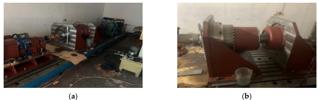
Figure 13. Installation diagram of the bench equipment: (a) horizontal test bench and (b) reducer clutch.
