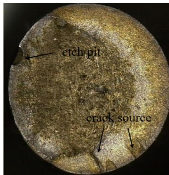
**Figure 12.** Corrosion fatigue fracture surface of 4330 sample.
