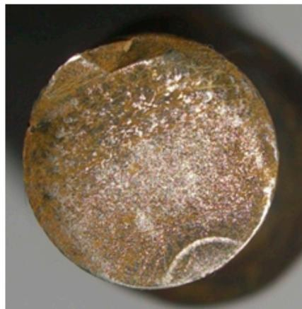
**Figure 6.** Fracture morphology of broken 4330 sucker rod in A well.
