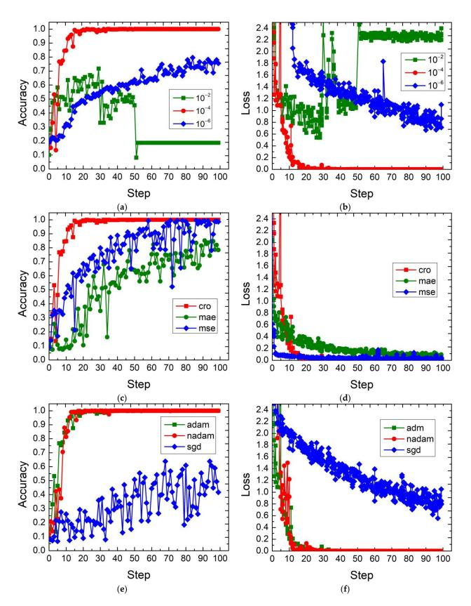
**Figure 10.** FSRCNN training accuracy and loss curves: (a) training accuracy with the learning rate; (b) training loss with the learning rate (cross entropy, nadam); (c) training accuracy with the loss function; (d) training loss with the loss function ( $lr = 10^{-4}$ , nadam); (e) training accuracy with the optimizer; (f) training loss with the optimizer ( $lr = 10^{-4}$ , cross entropy).
