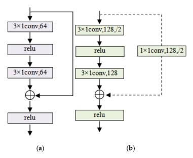
Figure 3. Residual convolution block: (a) identity residual block; (b) projection residual block.
