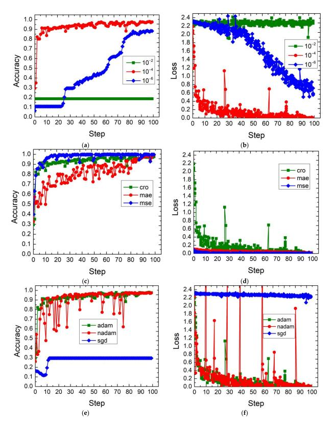
**Figure 9.** TSRCNN training accuracy and loss: (a) training accuracy with the learning rate; (b) training loss with the learning rate (cross entropy, nadam); (c) training accuracy with the loss function; (d) training loss with the loss function ( $lr = 10^{-4}$ , nadam); (e) training accuracy with the optimizer; (f) training loss with the optimizer ( $lr = 10^{-4}$ , cross entropy).
