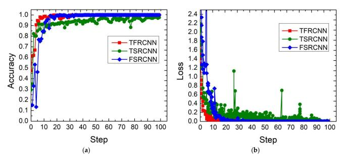
**Figure 11.** Optimized training accuracy and loss curves for TFRCNN, TSRCNN, and FSRCNN: (a) optimized training accuracy curves; (b) optimized training loss curves.
