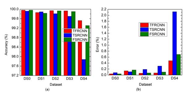
**Figure 14.** Mean accuracy and error of the models under a specific load: (**a**) mean accuracy; (**b**) mean error.
