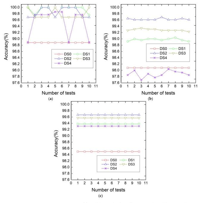
**Figure 16.** Accuracy of the models trained with DS4 for 10 repeated tests: (**a**) TFRCNN; (**b**) TSRCNN; (**c**) FSRCNN.
