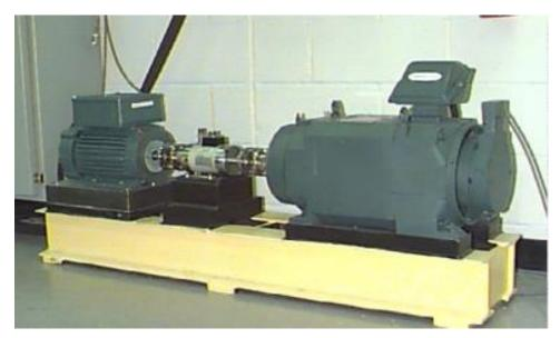
Figure 6. Rolling bearing test rig.
