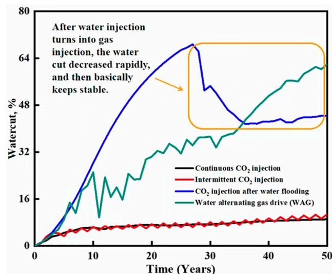
Figure 11. Watercut curves of four cases.
