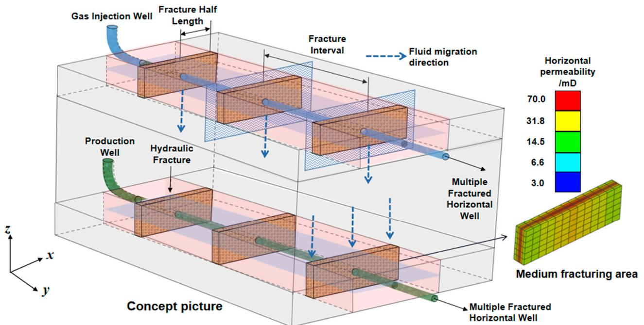
Figure 3. Low-permeability sandstone reservoir model with hydraulic fractures.
