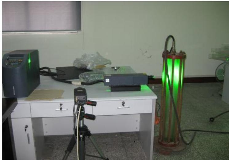
**Figure 2.** Irradiation experiment on compressed acrylic pipe.
