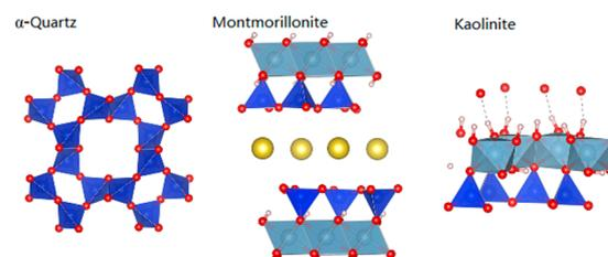
**Figure 2.** Crystal structure of  $\alpha$ -quartz, montmorillonite, and kaolinite.
