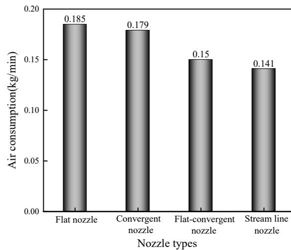
**Figure 6.** Comparison of air consumption of different nozzle shapes.
