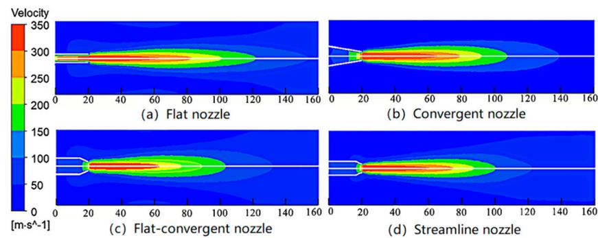
**Figure 4.** Nozzle jet velocity variation.
