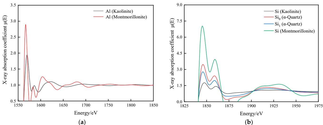
**Figure 3.** The X-ray absorption coefficients of Al and Si atoms in  $\alpha$ -quartz, montmorillonite, and kaolinite. (a) The absorption coefficient of Al atoms in kaolinite and montmorillonite; (b) the absorption coefficient of Si atoms in kaolinite,  $\alpha$ -quartz, and montmorillonite.
