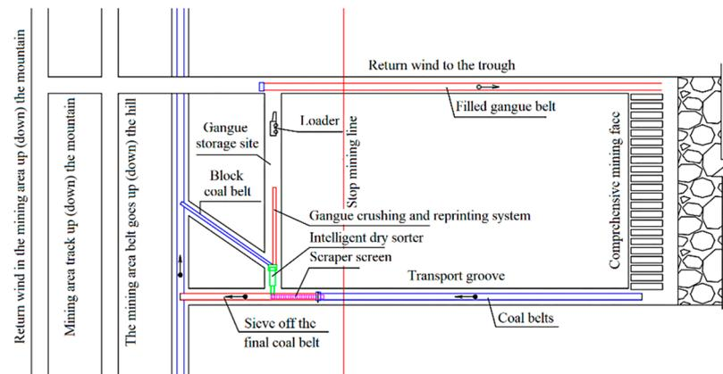
**Figure 10.** Haulage roadway distribution of distributed layout type.
