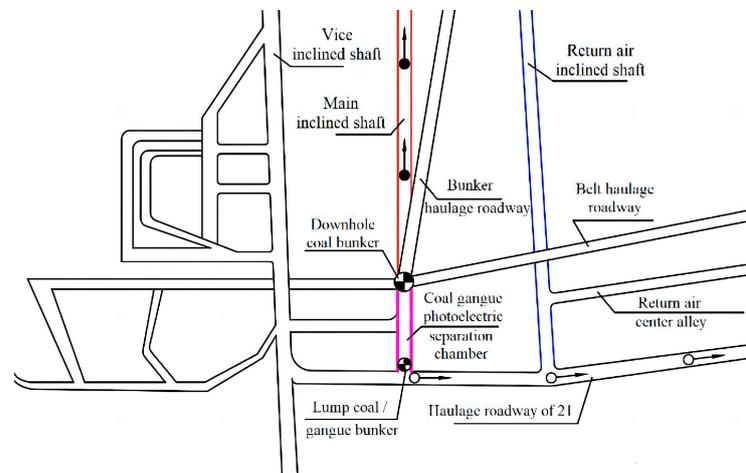
**Figure 8.** Haulage roadway distribution of centralized layout type.
