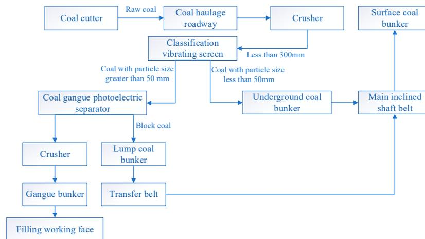
**Figure 7.** Technological process of underground coal gangue photoelectric separation system.
