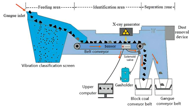
**Figure 1.** Schematic diagram of coal gangue photoelectric separation system.
