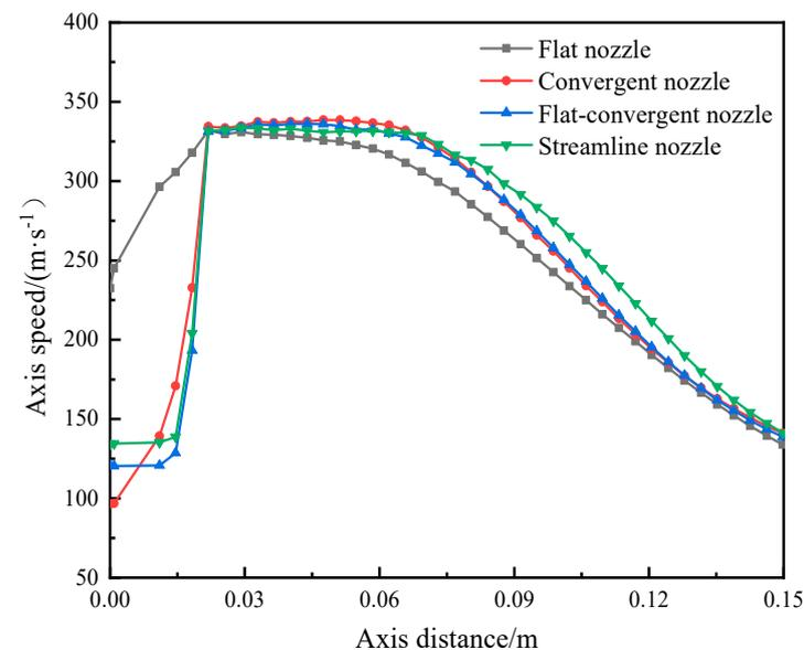
**Figure 5.** Comparison of nozzle axis speed of different shapes.
