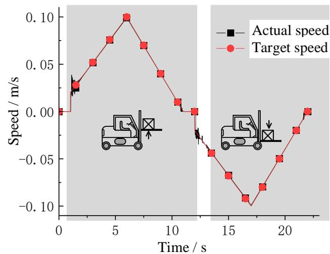
**Figure 8.** Cylinder speed curves under constant pressure-difference speed regulation.
