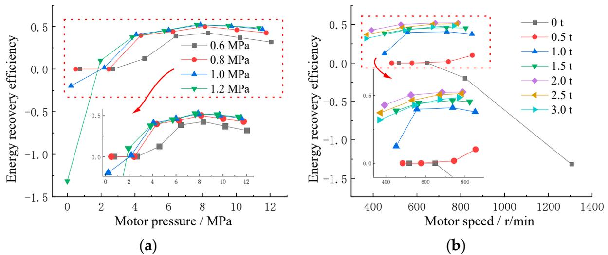
**Figure 20.** Energy-recovery efficiency test curves under different pressures and speeds during descending stage. (a) Energy-recovery efficiency vs. motor pressure; (b) energy-recovery efficiency vs. motor speed.
