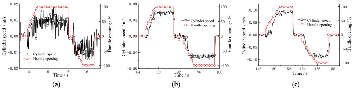
**Figure 18.** Cylinder speed test curves under different target pressure differences. (a) 0.1 MPa; (b) 0.8 MPa; (c) 1.6 MPa.
