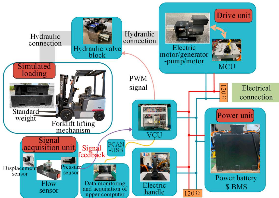
Figure 15. Electric forklift hydraulic system test bench.
