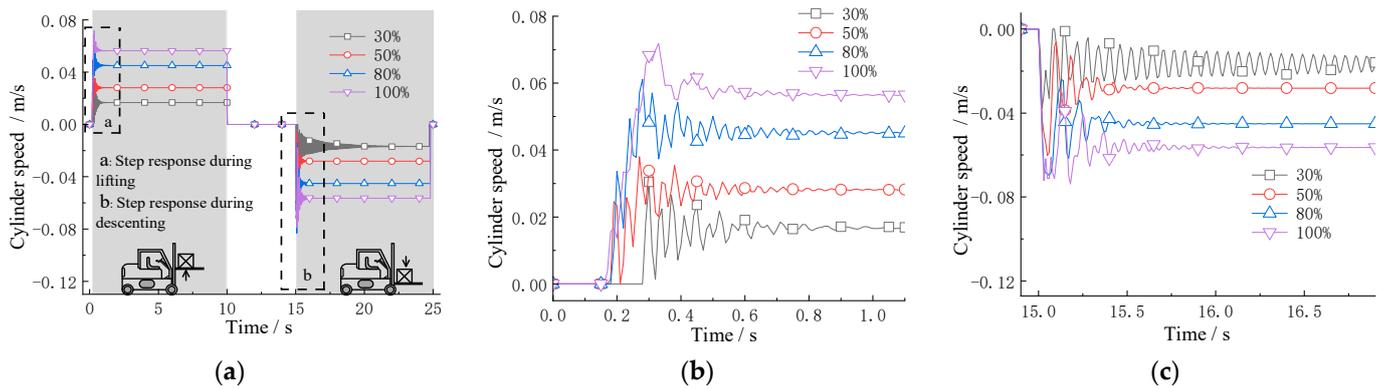
**Figure 12.** Cylinder speed curves under different valve openings. (a) Cylinder speed curves; (b) enlarged image of range a; (c) enlarged image of range b.
