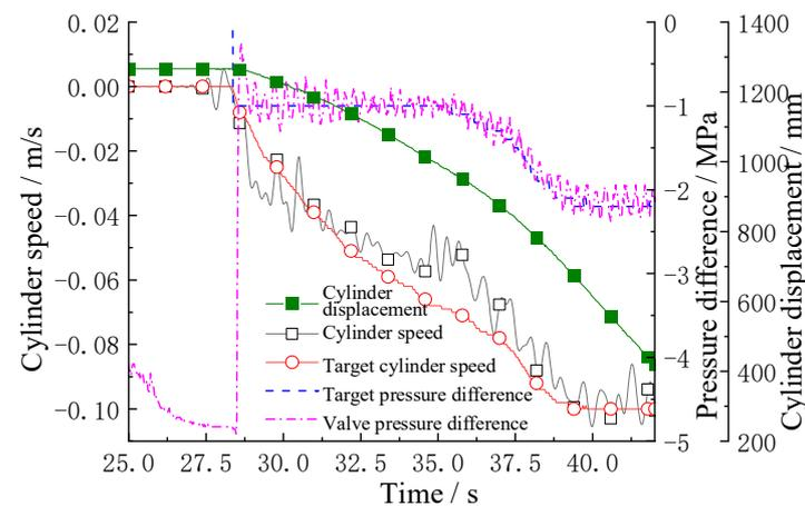
**Figure 22.** Variable pressure difference pump–valve compound speed control following ramp descending.
