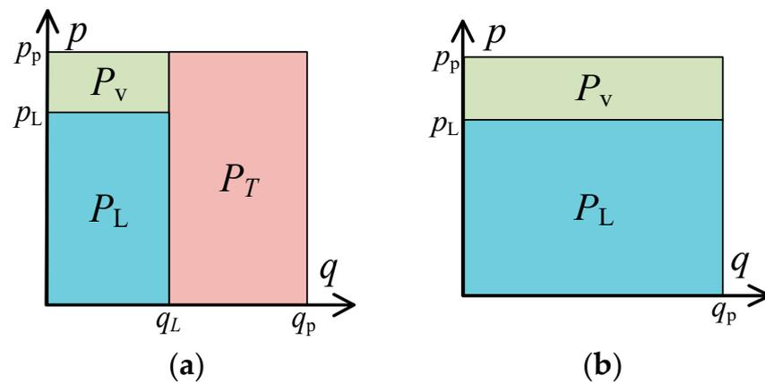
**Figure 3.** Diagram of energy consumption of traditional valve-controlled lifting. (a) Non-full speed; (b) full speed.
