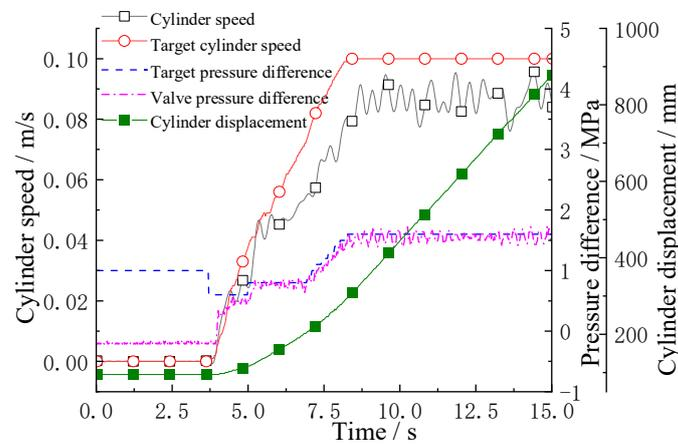
**Figure 21.** Variable pressure difference pump–valve compound speed control following ramp lifting.
