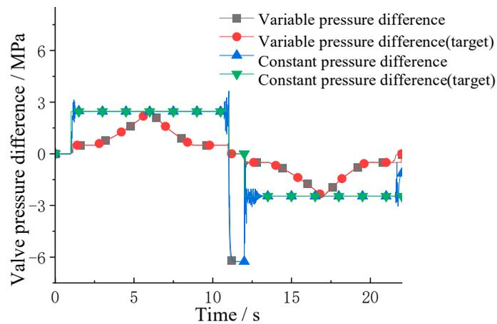
Figure 11. Curves of pressure difference across the valve.
