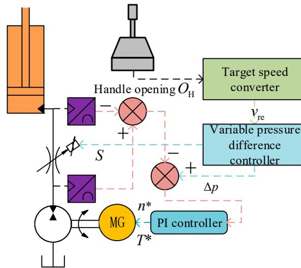
Figure 5. Variable pressure-difference pump–valve compound speed-regulation diagram.
