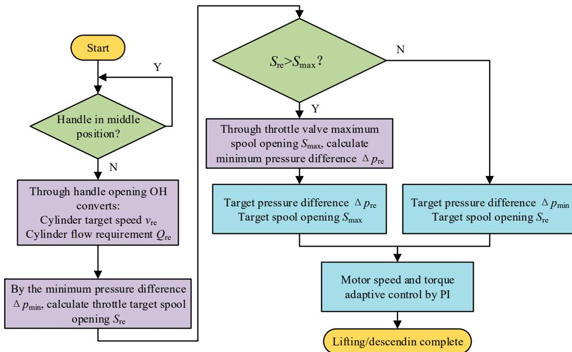
Figure 6. Variable pressure-difference pump–valve compound speed-regulation control strategy flowchart.
