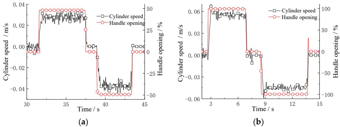
**Figure 16.** Cylinder speed test curves under different valve openings. (a) 50%; (b) 100%.
