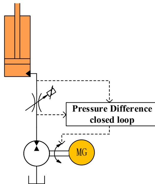
**Figure 4.** Throttling loss energy-regeneration system based on pressure difference pump control.
