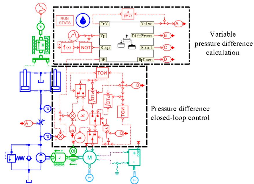
Figure 7. Simulation model of variable pressure difference pump–valve compound speed regulation.
