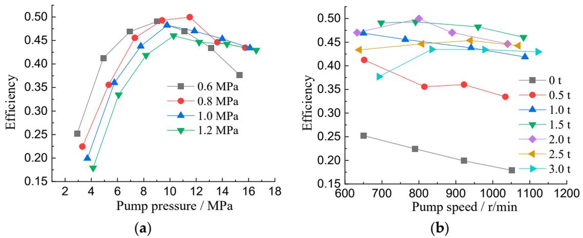
**Figure 19.** Total efficiency test curves under different pressures and pump speeds during lifting stage. (a) Efficiency vs. pump pressure; (b) efficiency vs. pump speed.
