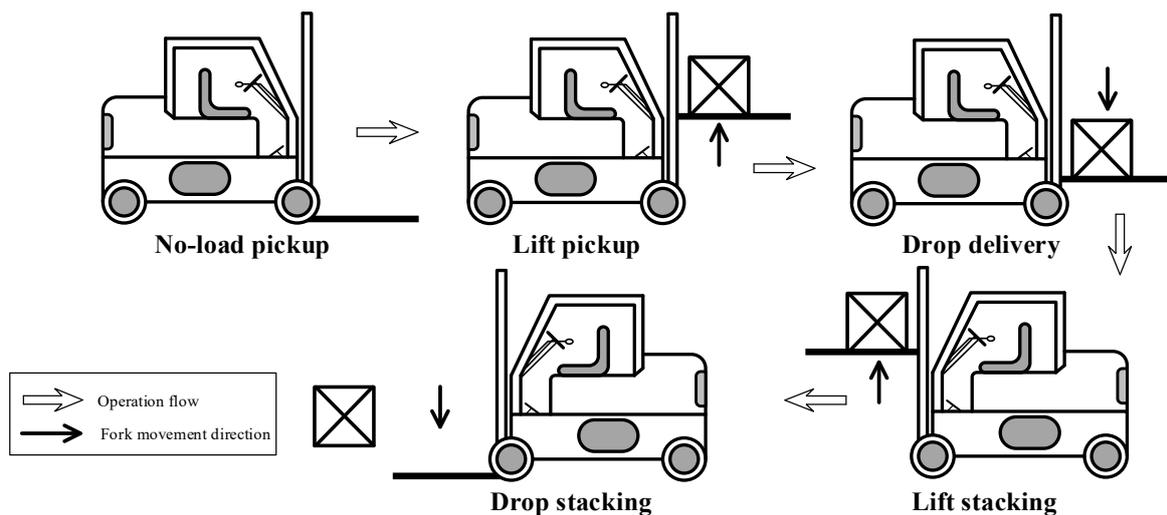
Figure 2. Forklift operation flowchart.
