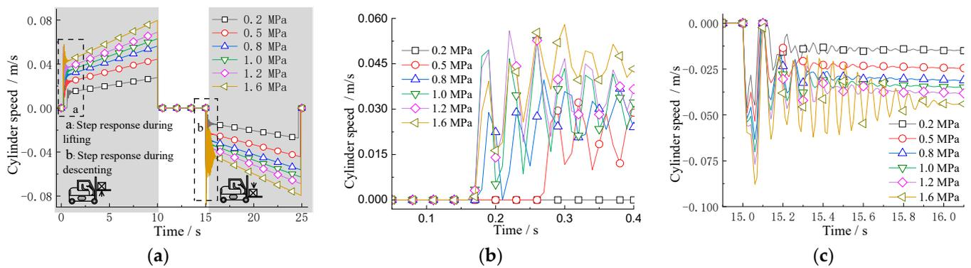
**Figure 13.** Cylinder speed curves under different target pressure differences. (a) Cylinder speed curves; (b) enlarged image of range a; (c) enlarged image of range b.
