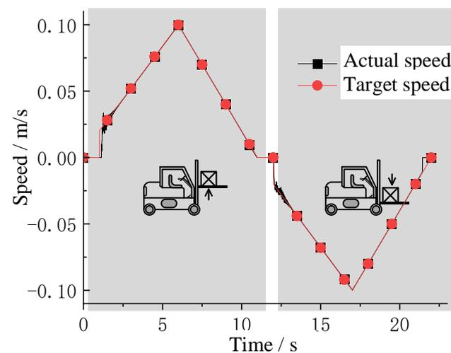
**Figure 9.** Cylinder speed curves under variable pressure-difference speed regulation.
