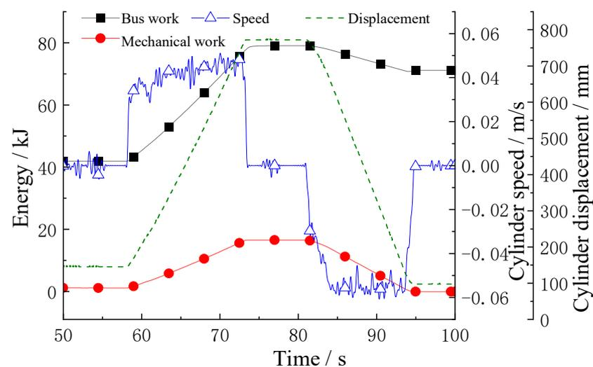
**Figure 23.** Energy-consumption curves of variable pressure-difference pump–valve compound speed-regulating system.
