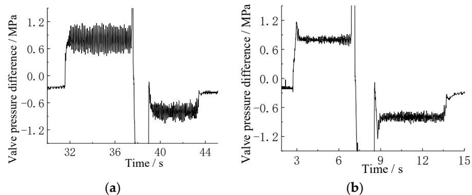
**Figure 17.** Throttle pressure-difference test curves under different valve openings. (a) 50%; (b) 100%.
