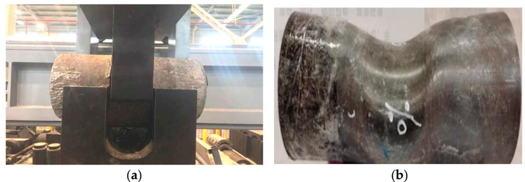
**Figure 11.** Test of full wellbore shear casing simulation: (a) simulation of casing under shearing; (b) features of casing after shear deformation.
